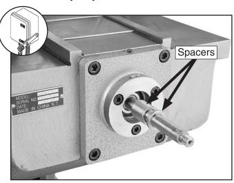
**Figure 69.** Ball handle and graduated dial removed from Y-axis lead screw.
