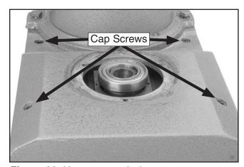
Figure 80. Upper transmission case cap screws.
