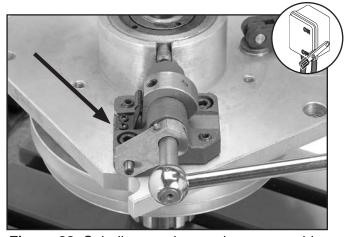
Figure 83. Spindle speed range lever assembly.
