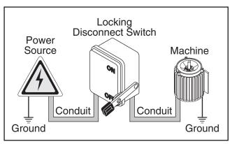
**Figure 4.** Typical setup of a permanently connected machine.
