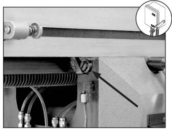
**Figure 65.** X-axis gib adjusting screw (underneath the left side of the table).
