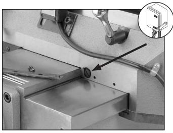
**Figure 66.** Y-axis gib adjusting screw (right front side of table).
