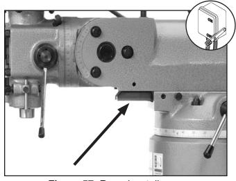
Figure 57. Ram dovetail way.
