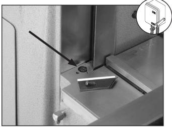
**Figure 67.** Z-axis gib adjusting screw (left side of knee).
