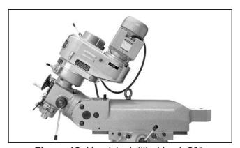
Figure 19. Headstock tilted back 30°.
