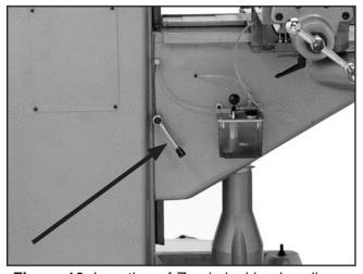
**Figure 16.** Location of Z-axis locking handle on left side of the knee.
