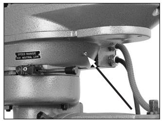
**Figure 64.** Model G9903 speed range gearing grease fitting.
