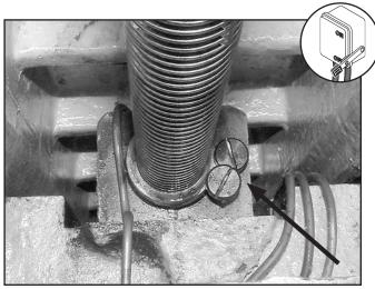
**Figure 68.** X-axis lead screw backlash adjusting screws.
