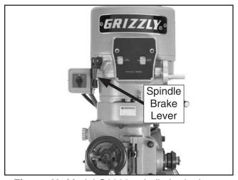
Figure 40. Model G9903 spindle brake lever.
