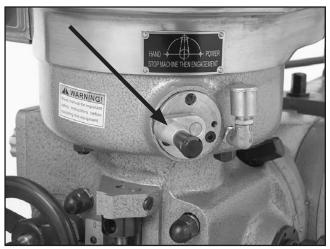
**Figure 34.** Manual/power downfeed selector in the manual or "hand" position.
