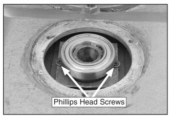
Figure 79. Upper spindle bearing.
