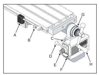
Figure 17. X-axis power feed system.
