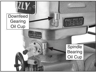
**Figure 53.** Model G9901/G9902 downfeed gearing and spindle bearing oil cups.
