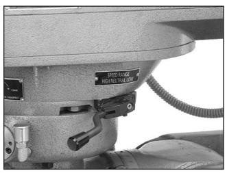
**Figure 29.** Model G9903 spindle speed range lever (shown in high range).
