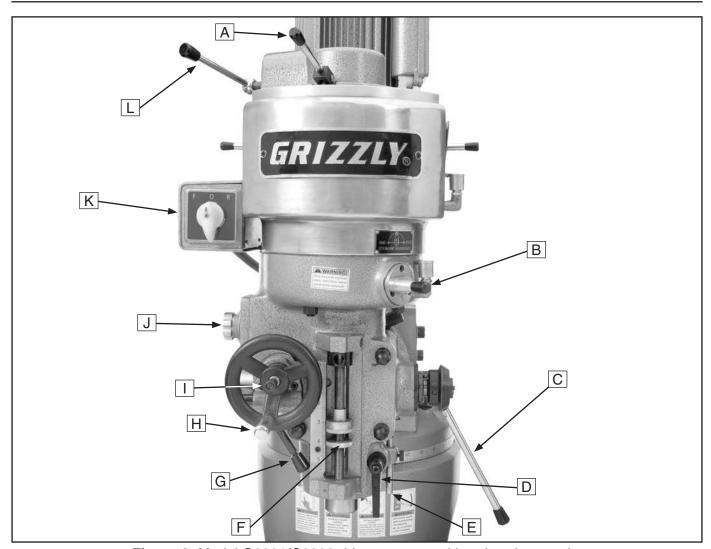
Figure 3. Model G9901/G9902 drive system and headstock controls.
