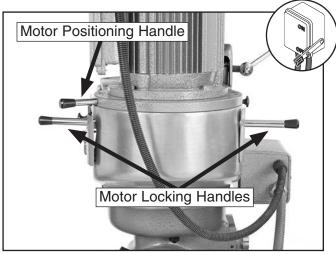
**Figure 31.** Model G9901/G9902 motor positioning controls (shown from rear of motor).
