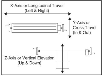
**Figure 13.** The three axis paths of the mill table travel.
