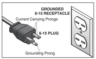
Figure 1. Typical 6-15 plug and receptacle.
