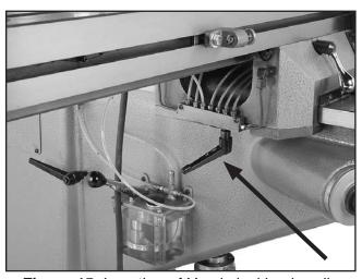
**Figure 15.** Location of Y-axis locking handle underneath the left side of the table.
