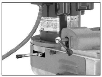
**Figure 28.** Model G9901/G9902 spindle speed range lever (shown in the low range).
