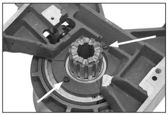
Figure 86. Pulley assembly screws.
