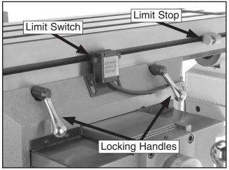
**Figure 18.** X-axis locking handles, limit stops, and limit switch.
