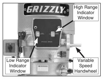
**Figure 33.** Model G9903 variable speed handwheel and speed indicator windows.
