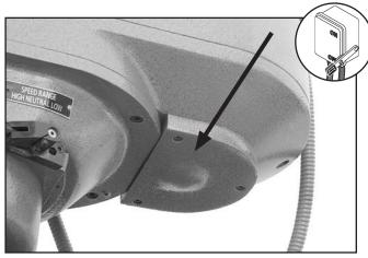
Figure 75. Lower pulley cover.
