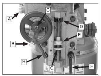
Figure 36. Fine and power downfeed controls.
