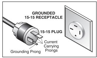
Figure 3. Typical 15-15 plug and receptacle.
