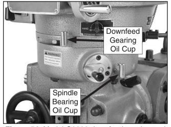
**Figure 54.** Model G9903 downfeed gearing and spindle bearing oil cups.
