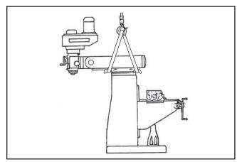
Figure 10. Using lifting straps to move the mill.
