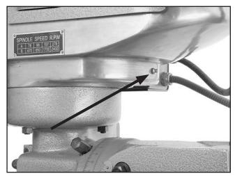
**Figure 63.** Model G9901/G9902 speed range gearing grease fitting.
