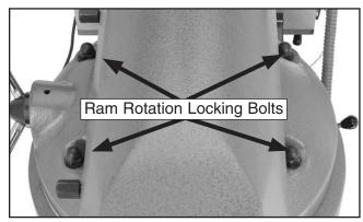
Figure 24. Ram rotation locking bolts.
