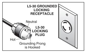
Figure 2. Typical L5-30 plug and receptacle.
