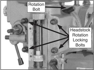
**Figure 22.** Headstock rotation locking bolts and rotation bolt.
