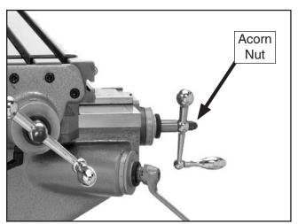
Figure 8. Table ball handle properly installed.
