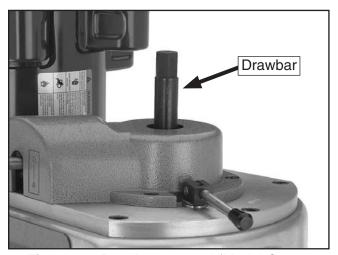
**Figure 42.** Drawbar inserted (Model G9902 shown).
