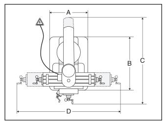
Figure 7. Model G9901/G9902/G9903 working dimensions.
