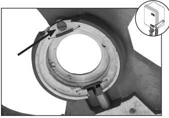
Figure 87. Brake shoe retaining screw.
