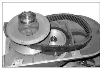
Figure 82. Variable speed belt.
