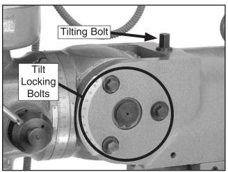
**Figure 21.** Headstock tilt locking bolts and tilting bolt.
