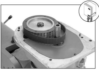
Figure 81. Ribbed timing belt.
