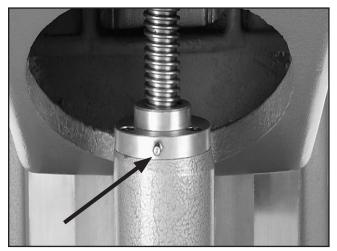
Figure 56. Elevation lead screw grease fitting.
