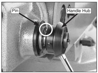
Figure 35. Coarse downfeed handle engaged.
