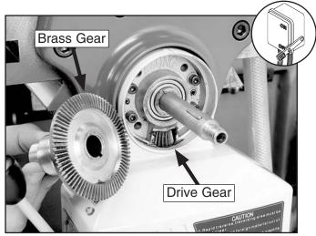
Figure 62. Power feed gears.
