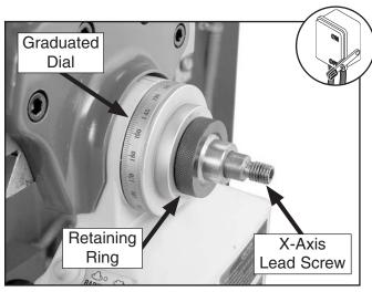
**Figure 60.** Power feed with the handwheel removed.
