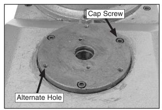
**Figure 78.** Upper bearing housing and cap screws.
