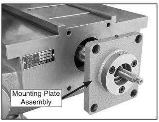
**Figure 70.** Removing mounting plate assembly from lead screw.
