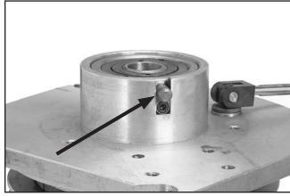
Figure 84. Gear change pin.
