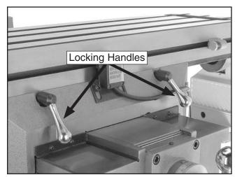
Figure 14. X-axis locking handles.
