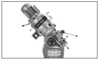
**Figure 20.** Headstock rotated to the right 45°.
