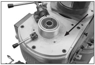
Figure 74. Transmission case cover plate.
