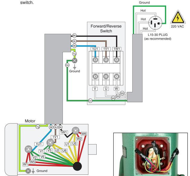
**Figure 91.** Model G9903 220V motor wiring.
