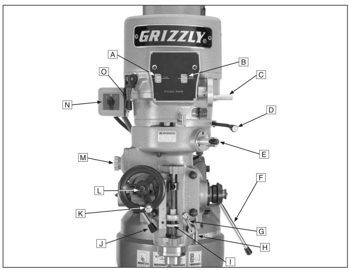
Figure 4. Model G9903 drive system and headstock controls.
