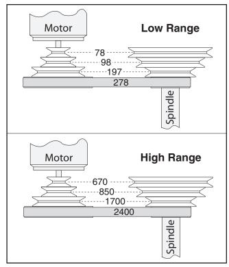
**Figure 32.** Model G9901/G9902 V-belt positioning for desired speed (RPM).
