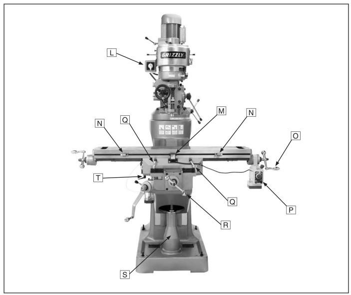
Figure 2. Identification, front (Model G9902 shown).
