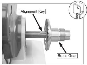
**Figure 61.** Power feed alignment key and brass gear.
