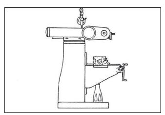
Figure 9. Using the eye bolt to lift the mill.
