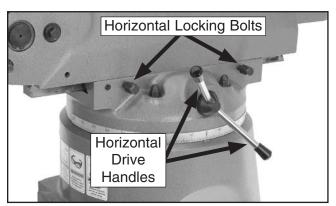
**Figure 23.** Ram horizontal locking bolts and drive handles.
