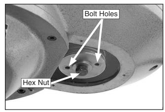
**Figure 76.** Location of the two spring retaining plate holes and hex nut.
