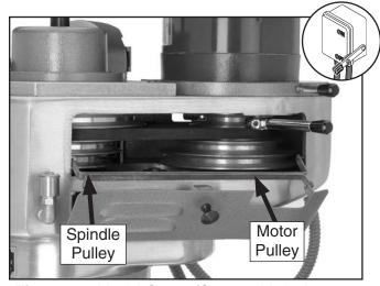
**Figure 30.** Model G9901/G9902 side belt cover removed (right side shown).
