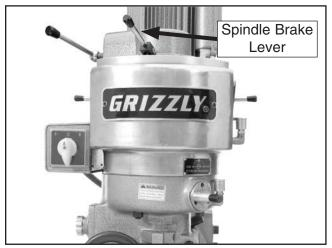
**Figure 39.** Model G9901/G9902 spindle brake lever.
