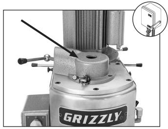
**Figure 58.** Model G9901/G9902 drawbar access.
