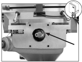
Figure 71. Y-axis lead screw adjusting screws.
