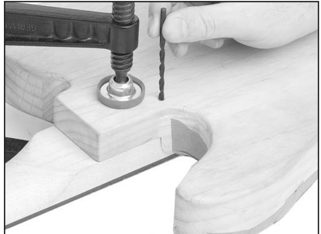
Figure 8. Making a pilot hole in the neck.
