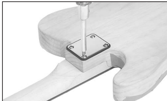
Figure 10. Fastening neck to body.
