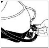
**Step 4** Connect the hose reel high pressure hose extension to the unit's high pressure outlet.
