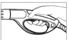
Step 3 Turn on the pressure washer. Pull trigger to operate unit: Liquid detergent is drawn into the unit and mixed with water. Apply detergent to work area. Do not allow detergent to dry on surface.
