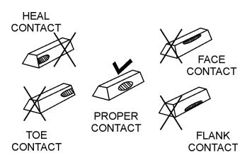
Figure 31. Gear Teeth Alignment
