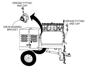
Figure 27. Grease Fittings (Dumping Mechanism)
