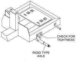
Figure 35. Axle Support Components
