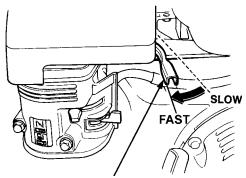
THROTTLE LEVER Figure 13. Throttle Lever
