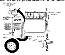
Figure 26. Grease Fittings (Drum Head Seals)
