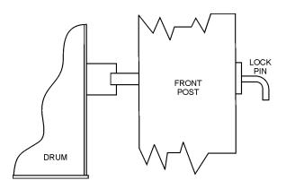
Figure 17. Drum Lock Pin (Side-View)
