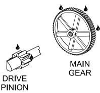
Figure 32. Pinion and Bull Gear Lubrication
