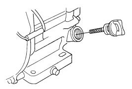
Figure 9. Engine Oil Dipstick (Removal)
