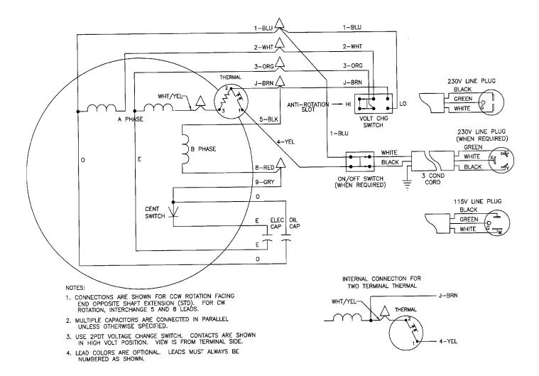
Figure 38. Electric Motor Wiring Diagram
