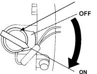
Figure 14. Engine ON/OFF Switch
