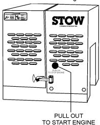
Figure 15. Start/Stop Switch (gasoline engine)
