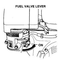
Figure 11. Fuel Shut-OFF Lever
