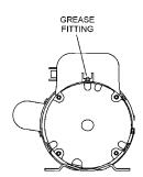
Figure 33. Grease Fittings Electric Motor
