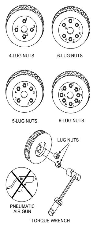
Figure 34. Wheel Lug Nuts Tightening Sequence
