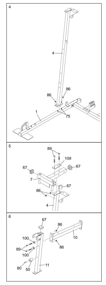
Slide the Butterfly Leg (11) onto the two M8 x 61mm Carriage Bolts (75) in the Butterfly Base (1). Hand tighten two M8 Nylon Locknuts (86) onto the Bolts. **Do not tighten the Locknuts yet.**
