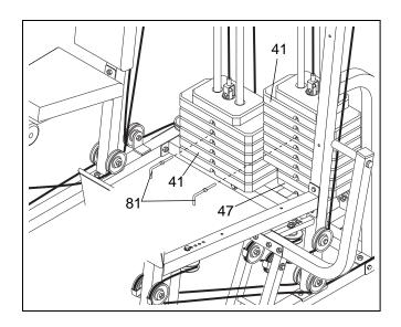
Note: Due to the cables and pulleys, the amount of resistance at each exercise station may vary from the weight setting. Use the WEIGHT RESISTANCE CHART on page 27 to find the approximate amount of resistance at each weight station.
