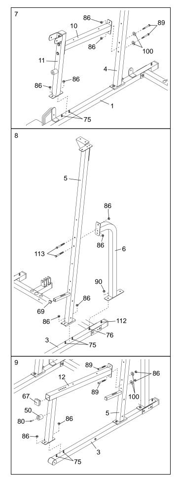
10. Press a 50mm Square Inner Cap (67) into the Press Top Frame (9).
