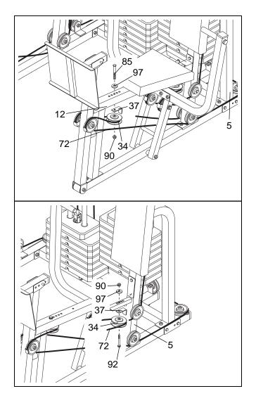
If a cable slips off the pulleys often, the cable may have become twisted. Remove the cable and re-install it. If the cables need to be replaced, see ORDERING REPLACEMENT PARTS on the back cover of this manual.
