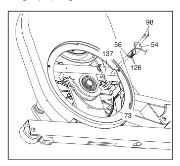
Next, remove the two M4 x 16mm Screws (98), and then remove the Reed Switch Bracket (54). Then, loosen, but do not remove, the two M4 x 10mm Clamp Screws (126).
