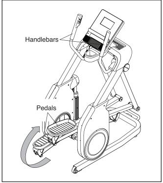
To dismount the elliptical, wait until the pedals come to a complete stop. Note: The elliptical does not have a free wheel; the pedals will continue to move until the flywheel stops. When the pedals are stationary, step off the higher pedal first. Then, step off the lower pedal.
