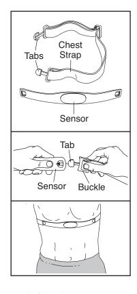
up. Then, attach the other end of the chest strap to the sensor. Adjust the length of the chest strap, if necessary.
