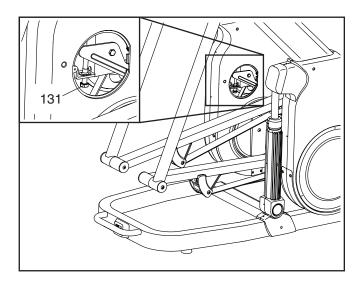
When you have properly adjusted the drive belt, reattach the access cover to the right inner shield.
