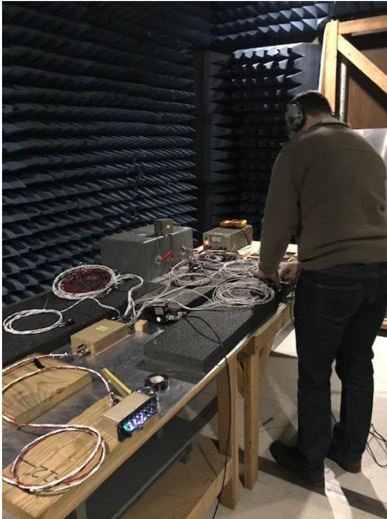
Figure 26 Emissions and susceptibility testing
