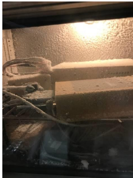
Figure 1 -Ground Survival Low Temperature and Short Term Operating Low temperature test
