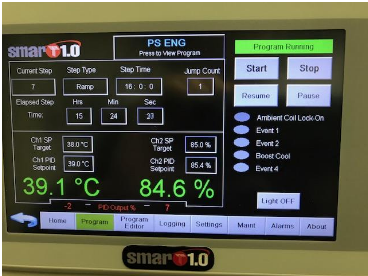
Figure 8 PAC45-SYSTEM System EUT Humidity tests
