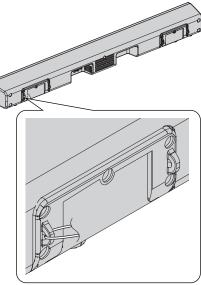
Loop the safety wires (not supplied) into each hole as shown and tie the safety wires to the LCD TV stand.
