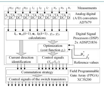
Figure 4. Control circuit basic schema.
