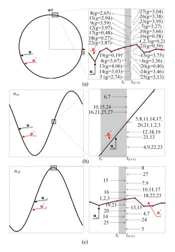
**Figure 5.** Example of the space vector geometrical interpretation for output reference  $u_o^*$  and obtained  $u_o$  voltages of the CSMC, a) vector locus, b)  $\alpha$  coordinates, c)  $\beta$  coordinates. (No. 1 to 27-*x*-SC number).
