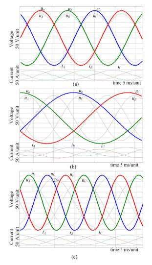
**Figure 7.** Simulation input voltages  $(u_A, u_B, u_C)$ , output voltages  $(u_a, u_b, u_c)$  and input currents  $(i_A, i_B, i_C)$  for reference output voltage amplitude 260 V and frequency (a) 50 Hz, (b) 25 Hz, (c) 75 Hz.
