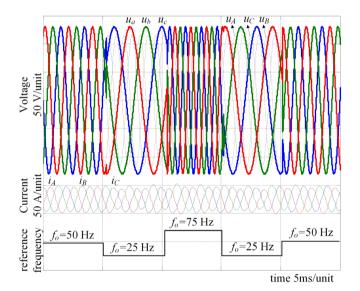
**Figure 9.** Simulation time waveforms of the input  $(u_A, u_B, u_C)$ , output  $(u_a, u_b, u_c)$  voltages and input currents  $(i_A, i_B, i_C)$  for variable output voltage frequency  $f_o$ .
