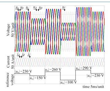
**Figure 8.** Simulation time waveforms of the input  $(u_A, u_B, u_C)$ , output  $(u_a, u_b, u_c)$  voltages and input currents  $(i_A, i_B, i_C)$  for variable reference output voltage amplitude  $|u_o|$ .
