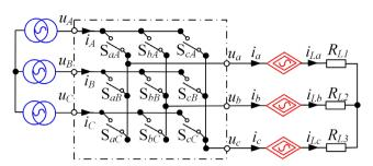
Figure 1. Simplified topology of current source matrix converter.
