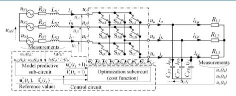
Figure 2. Simplified block scheme of the current source matrix converter with model predictive control circuit.
