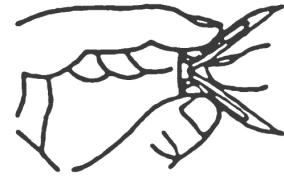
Fig. 17 - Folding the Expansion Bracket
