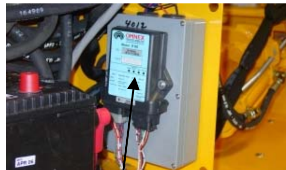
COMPARE THE LIGHT CONFIGURATION ON THE RECEIVER TO THE DIAGNOSTIC CHART IN THE RADIO CONTROL MANUAL
