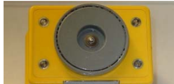
REMOVE THE BACK COVER TO ACCESS THE BATTERIES – THERE ARE 4 SCREWS HOLDING IT IN PLACE. THE BATTERY COMPARTMENT IS LABELED FOR CORRECT BATTERY ORIENTATION.
