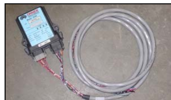
THE RADIO CONTROL RECEIVER, SHOWN AT THE RIGHT, MUST BE INSTALLED IN THE CONTROL BOX
