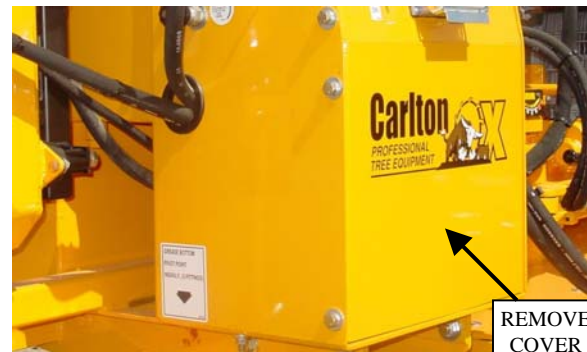
REMOVE THE BACK COVER TO ACCESS THE BATTERIES – THERE ARE 4 SCREWS HOLDING IT IN PLACE. THE BATTERY COMPARTMENT IS LABELED FOR CORRECT BATTERY ORIENTATION.
