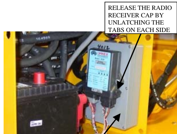
REMOVE THE REMOTE COVER TO ACCESS THE RADIO RECEIVER UNIT
