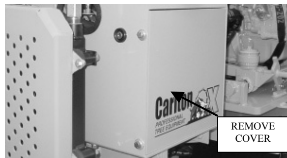
REMOVE THE BACK COVER TO ACCESS THE BATTERIES - THERE ARE 4 SCREWS HOLDING IT IN PLACE. THE BATTERY COMPARTMENT IS LABELED FOR CORRECT BATTERY ORIENTATION.
