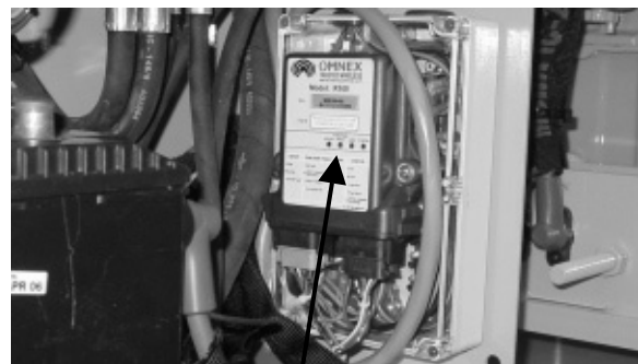
COMPARE THE LIGHT CONFIGURATION ON THE RECEIVER TO THE DIAGNOSTIC CHART IN THE RADIO CONTROL MANUAL
