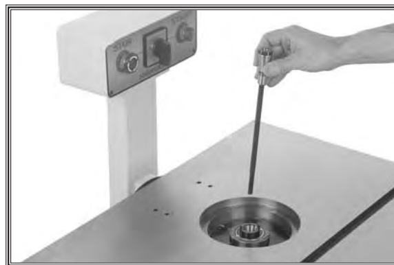
Figure 26. Inserting collet assembly into spindle cartridge.
