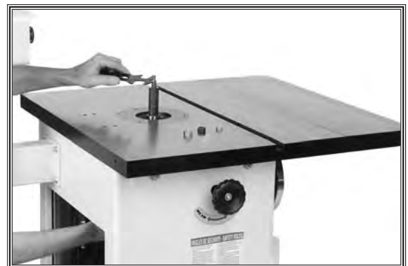
Figure 21. Final tightening drawbar nut and spindle.
