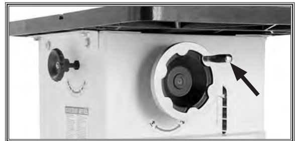
Figure 8. Handle installed in handwheel.
