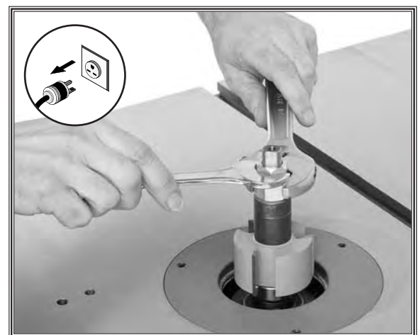
Figure 25. Tightening spindle nut.
