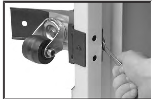
Figure 3. Installing caster (A).
