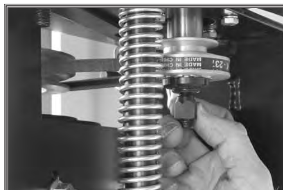
Figure 27. Tightening drawbar nut, taper side up.
