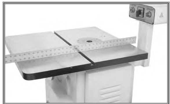
Figure 7. Checking overall table flatness with a straightedge.
