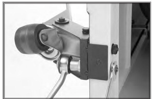
Figure 4. Installing caster (B).
