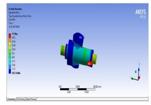
Fig 10: Equivalent (von-mises) stress at 60kN load
