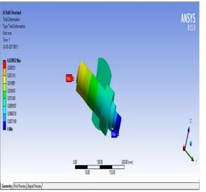
Fig 7: Total deformation at 40KN load
