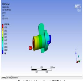
Fig 9: Total deformation at 50KN load
