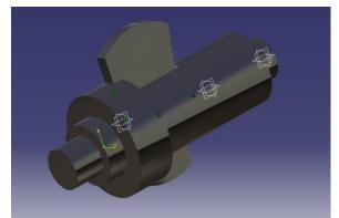
Fig 3: Assembly of cotter joint
