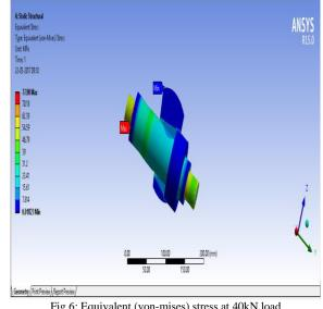
Fig 6: Equivalent (von-mises) stress at 40kN load
