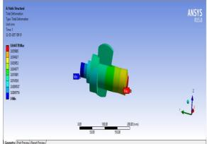
Fig 11: Total deformation at 60KN load
