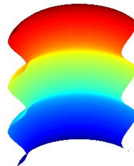
Fig. 2 A sweep surface generated from a pure rotation.
