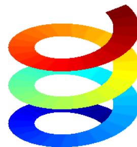
Fig. 3 A sweep surface generated from a combined translation and rotation.
