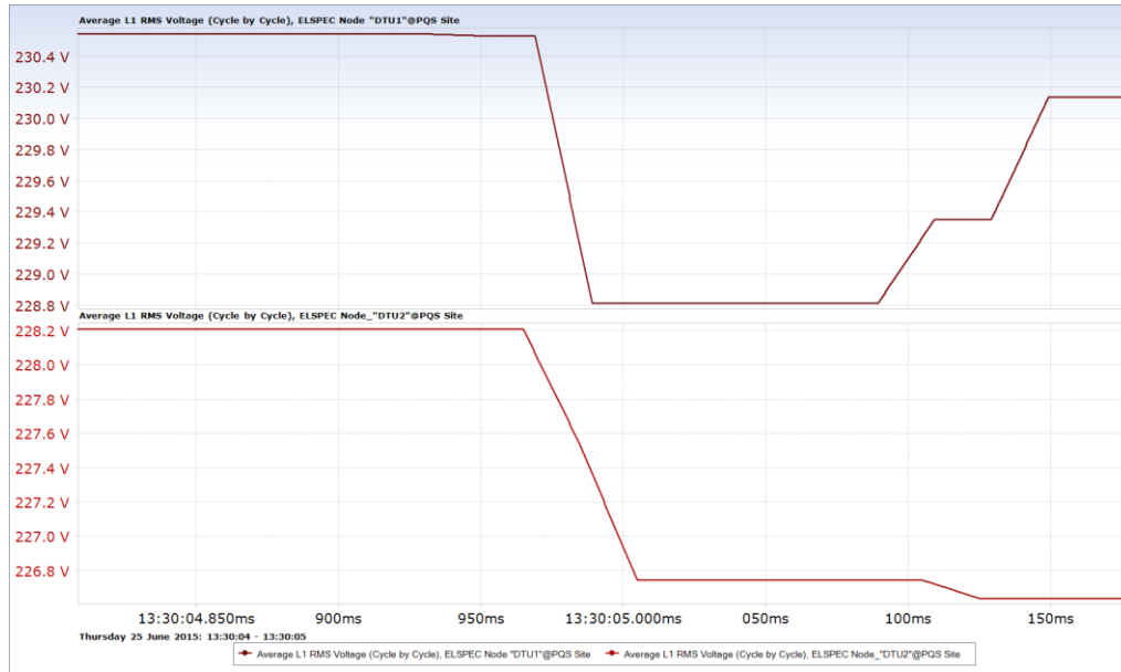
Fig. 31. Zoom-in of the phase-neutral voltage on phase a
