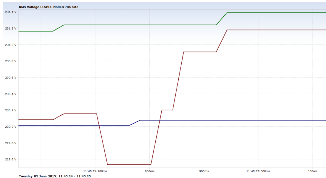
Fig. 28. 11:45 – Event #4: zoom-in of the phase-neutral voltage on phase a
