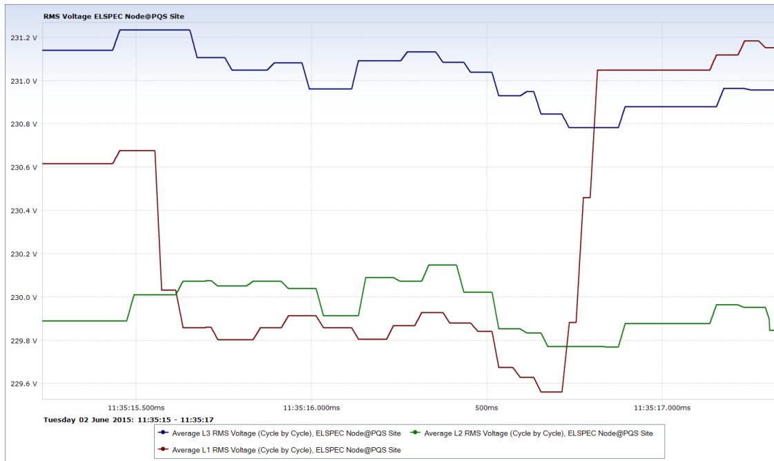
Fig. 23. 11:35 – Event #2: zoom-in of the phase-neutral voltage on phase a
