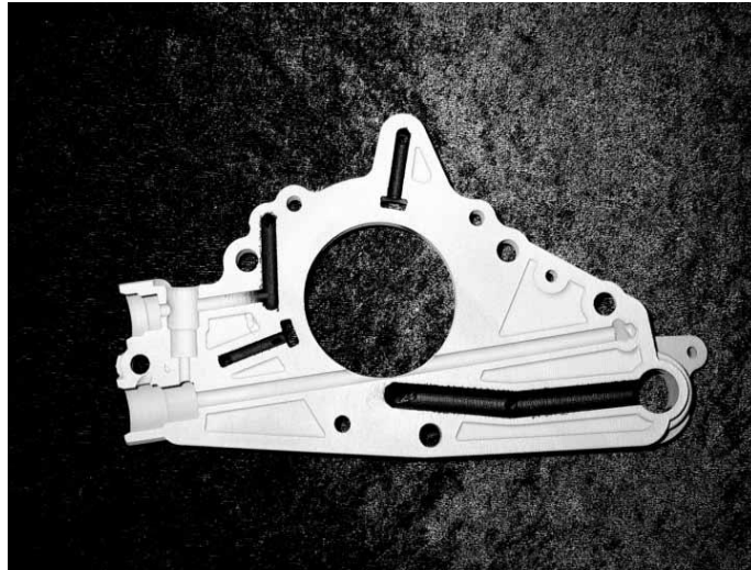
Figure 2.16: Sectional view of laser sintered part
