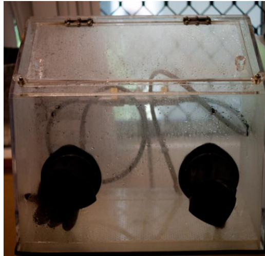
Figure 4.2: Water pressure apparatus for removing support structures
