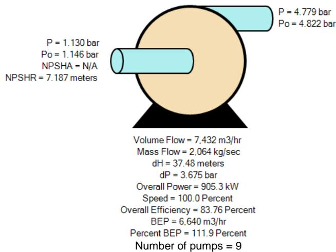
Figure 12 – Case D4 results for second pumping system
