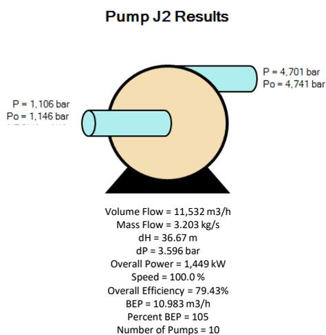
Figure 2 – Case D1 results for the pumping system
