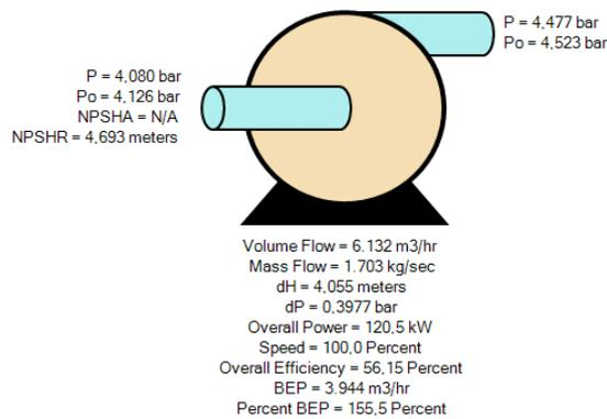
Figure 8 – Case D3 results for the auxiliary pumping system
