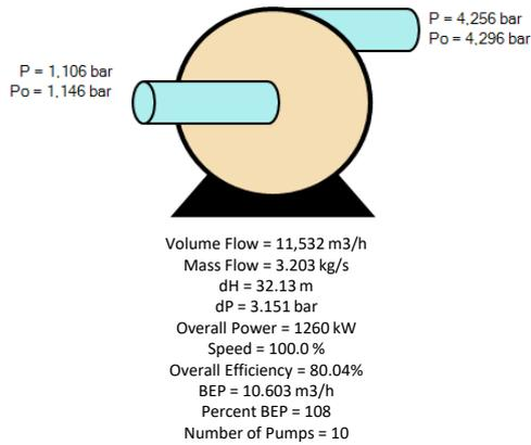
Figure 7 – Case D3 results for the main pumping system
