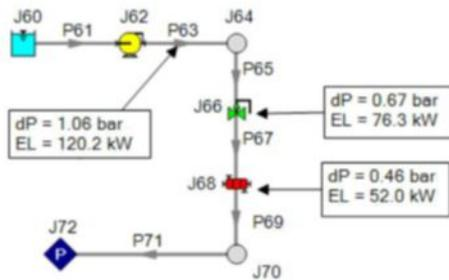
Figure 9 – Case D4 layout and results for first distribution system
