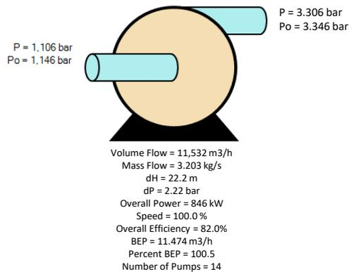
Figure 4 – Case D2 results for main pumping system
