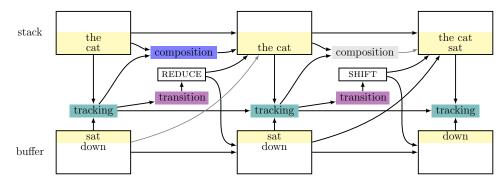
(a) The SPINN model unrolled for two transitions during the processing of the sentence *the* cat sat down. Tracking, transition, and composition are neural network layers. Gray arrows indicate connections which are blocked by a gating function.
