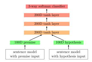
Figure 6.1: The neural network classification architecture: for each sentence-encoding model evaluated in Tables 6.3 and 6.4, two identical sentence encoders process the two input sentences and supply the 100D inputs shown here.
