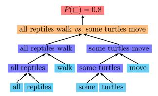
Figure 3.1: In the model evaluated in this chapter, based on the architecture in Section 2.3.4, two separate tree-structured networks (blue and lavender) build up vector representations for each of two sentences using either NN or NTN layer functions (lavender). A comparison layer (orange) then uses the resulting vectors to produce features for a classifier (red).
