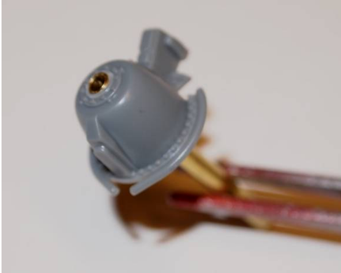
Brass tube in crankcase.
