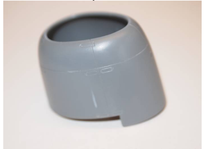
Picture of cowl sink mark repair.
