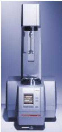
MCR 502 Rotation and oscillation tests for viscoelastic properties
