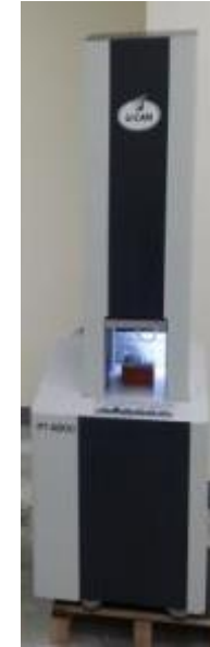
PT-6800 Specific volume with curing (PVTC)
