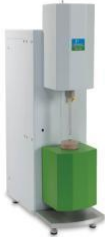
TMA 4000 Coefficient of thermal expansion
