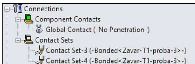
Figure 8: Defining contact sets between bodies
