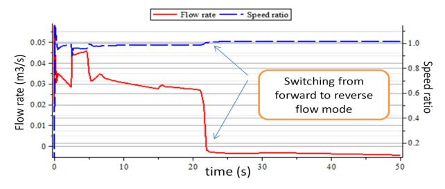
Figure 11: Torque converter flow rate and speed ratio during forward and reverse modes
