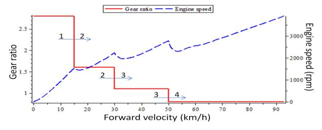
Figure 7: Engine speed and gear ratio variations
