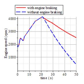
Figure 12: Engine braking effect on rpm
