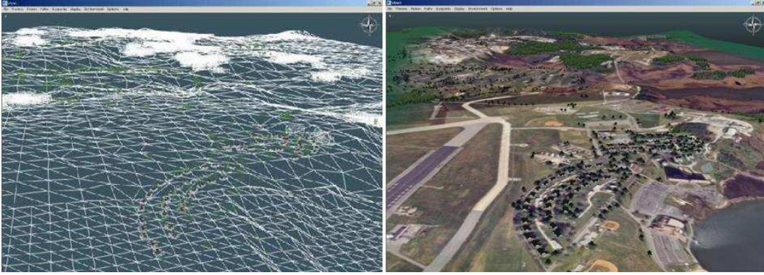
Figure 4.4: A wire-frame representation of a single DIRSIG object used to construct scenes
