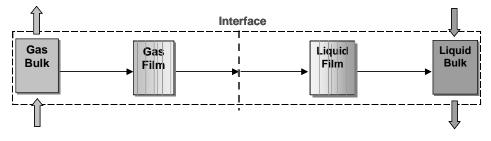
Figure 1. Schematic of the rate-based stage model
