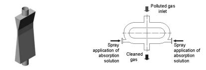
Figure 6. Venturi scrubber for flue gas cleaning Figure 7. O-Element for flue gas cleaning
