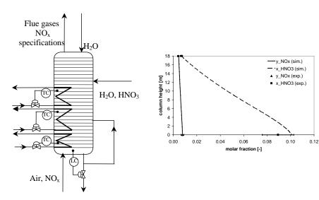
Figure 4. Reactive absorption for HNO<sub>3</sub> production
