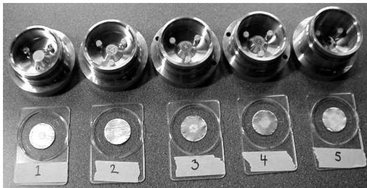
Figure 2-5 The impactor stages that were used in the particle size measurements and foils with deposits.
