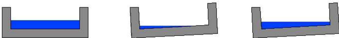
Figure 13. Situations of discharge spillage: rectangular, triangular and trapezoidal wetted area
