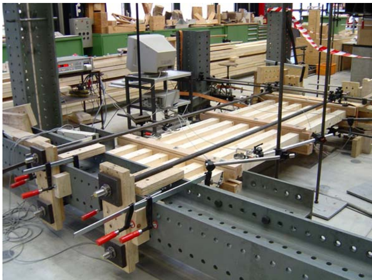
Figure 23: Shearing test of the proposed wall at EPFL-IBOIS (photo: T. Shiratori).
