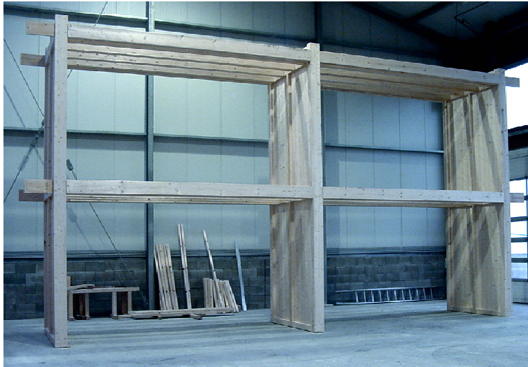
Figure 25: 2-storey frame tested by K. Tavoussi et al. at TUWien – ITI.
