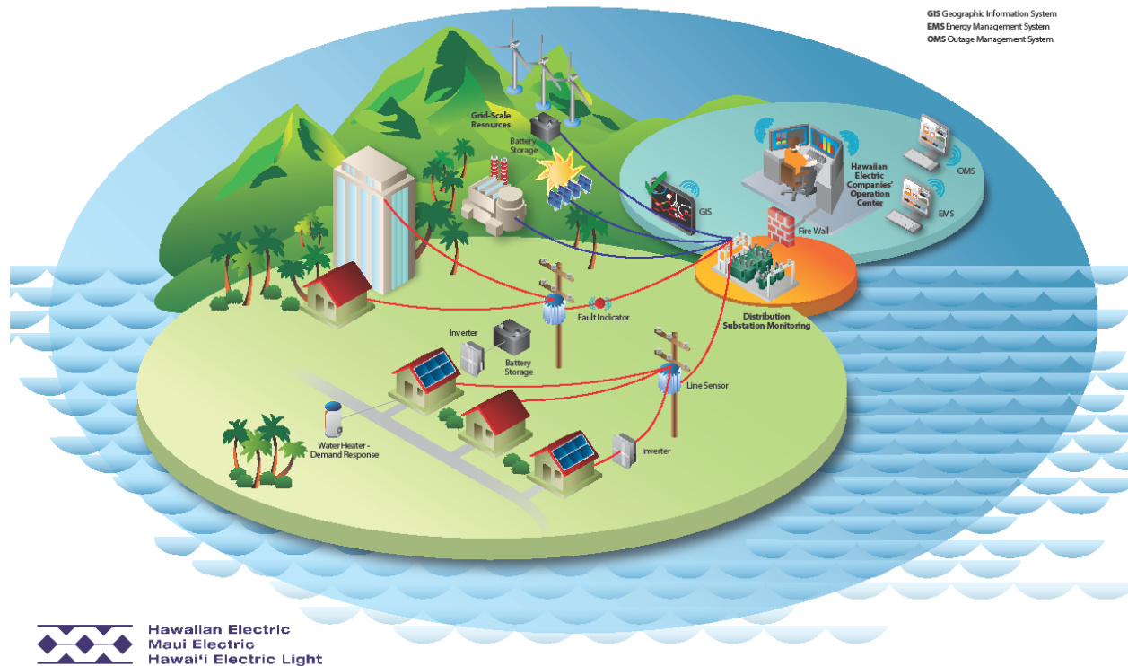
Figure 5 "Walk" - Depicting Current Technology Deployment on the Grid
