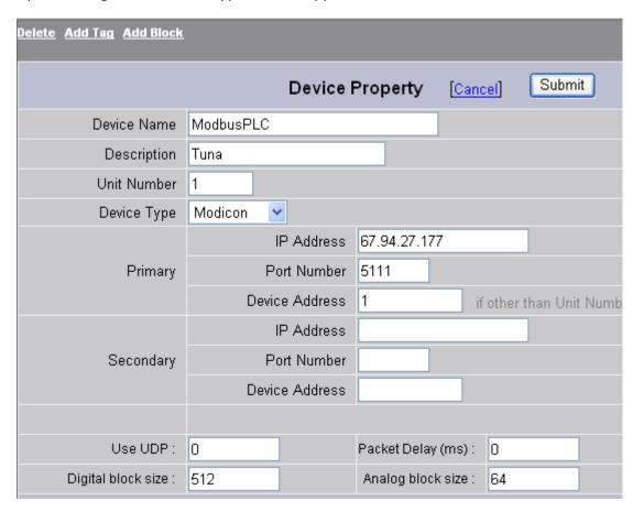
Figure 3-12Modicon - Modbus TCPIP device
