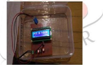
Figure 3.4 Temperature and Humidity measuring device
