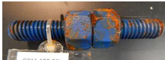
Figure 6: Condition of PTFE Sample after 840 hours salt fog
