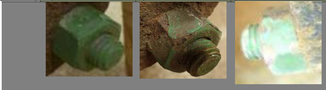
Figure 10: Field Trial Time Progression: Cd/PTFE
