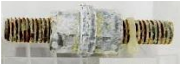
Figure 9: Hot Dipped Galvanized Sample after 50 Cycles
