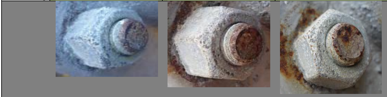
Figure 11: Field Trial Time Progression: HDG
