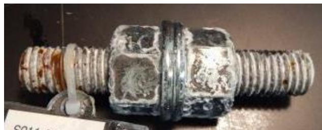
Figure 7: Condition of Electrogalvanized Sample after 168 hours salt fog.
