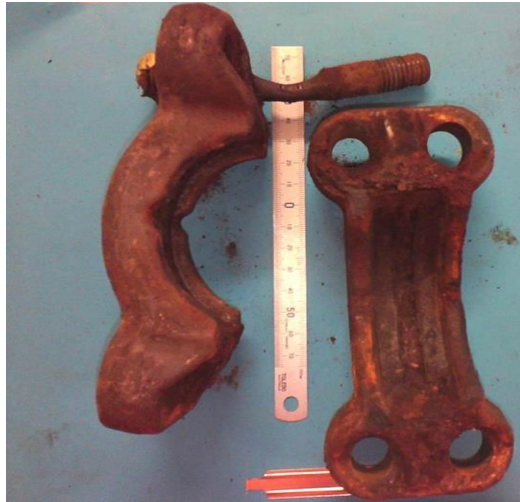
Figure 1: Example of Bolt Corrosion
