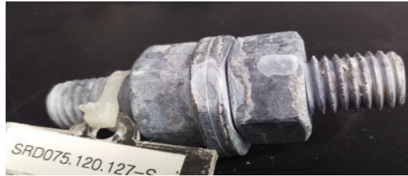
Figure 5: Condition of Zinc-nickel Nanolaminate Sample after 4000 hours salt fog.
