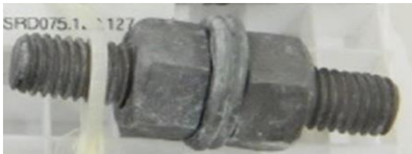
Figure 8: Zinc-nickel Nanolaminate Sample after 50 Cycles
