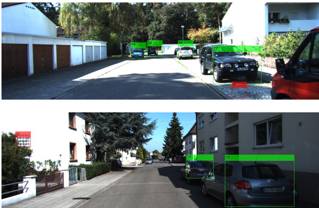
Figure 6: Results for vehicle detection tested on KITTI image frames, true positive detection (Green), false positive detection (Red)
