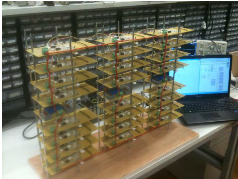
Fig. 7.5: Prototype of a 5-level MMC with embedded lithium-ion batteries.
