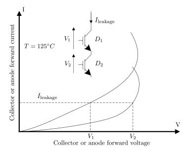
Figure A.1. Collector forward blocking I-V characteristics of two series devices.
