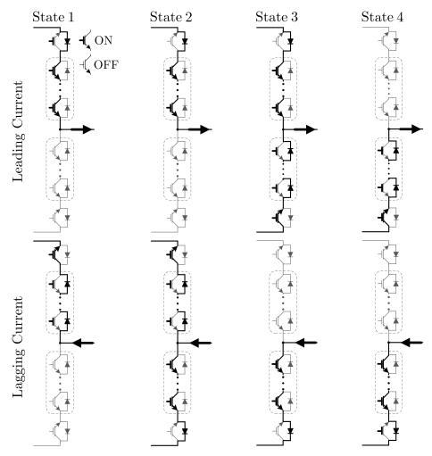
Figure 2.6. Description of zero-crossing transition in FBU.
