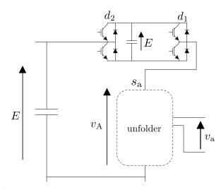
Figure 5.3. The schematic diagram of 5-level single-phase converter.
