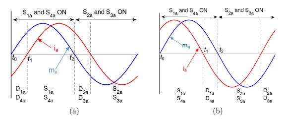
Figure 2.10. Unfolder transition (a) lagging current (b) leading current.
