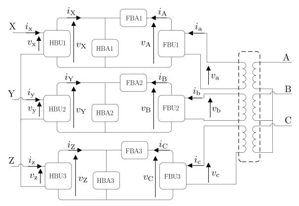
Figure 2.2. Schematic diagram of a three-phase SMMC.
