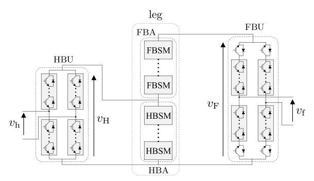
Figure 1.12. Single-phase sparse modular multilevel converter.
