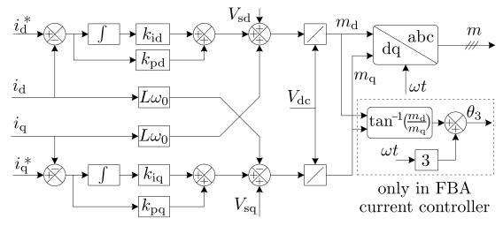
Figure 2.26. The schematic diagram of the current controller.
