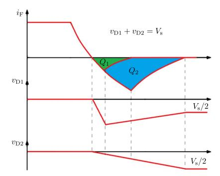
Figure A.3. Reverse recovery current and voltage for two mismatched series devices.
