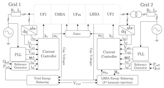
Figure 3.9. The schematic diagram of control strategy.
