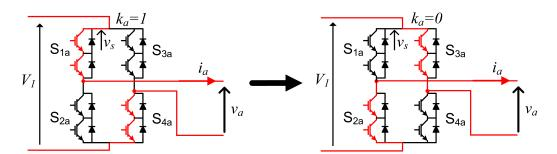
Figure 2.9. Schematic diagram of HBU switching transition.
