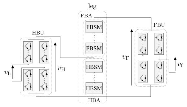
Figure 2.1. Schematic diagram of a single-phase *n*-level SMMC.
