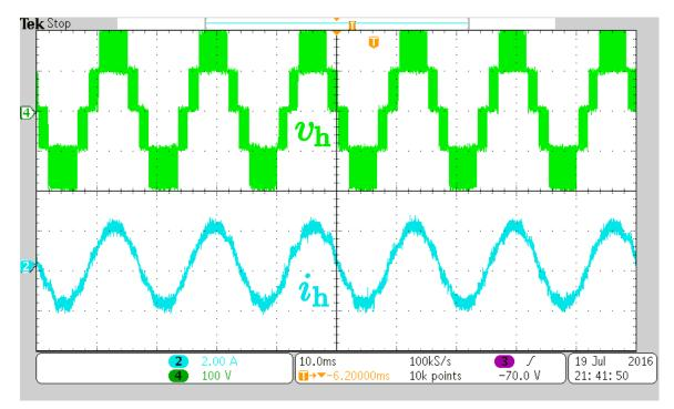
Figure 2.34. Converter's HB-side waveforms in steady-state condition.
