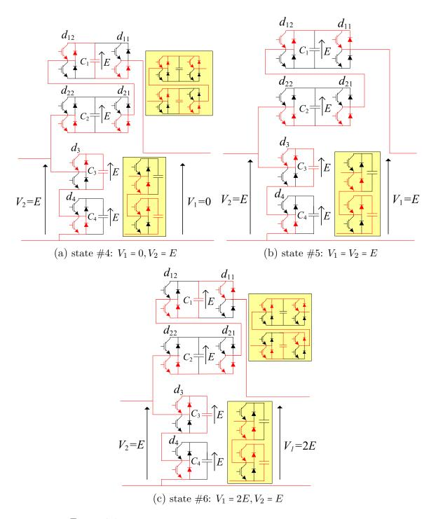
Figure 2.8. Illustration of switching states 4-6 in a 5-level SMMC
