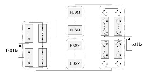
Figure 2.12. One phase of unidirectional SMMC with diode-bridge front unfolder.
