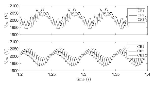
Figure 2.31. Average HBA and FBA capacitor voltages.
