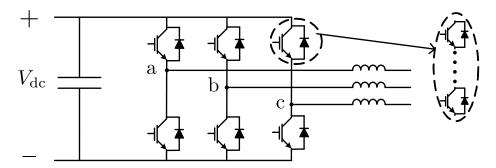
Figure 1.2. Schematic diagram of a 2-level high power voltage source inverter.
