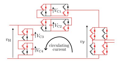
Figure 2.4. Zero-crossing circulating current in 5-level SMMC.
