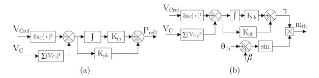
Figure 3.11. (a) Total energy balancing unit (b) LHBA energy balancing unit.
