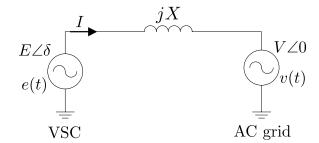
Figure 5.6. Simplified single-line diagram of converter-grid circuit.
