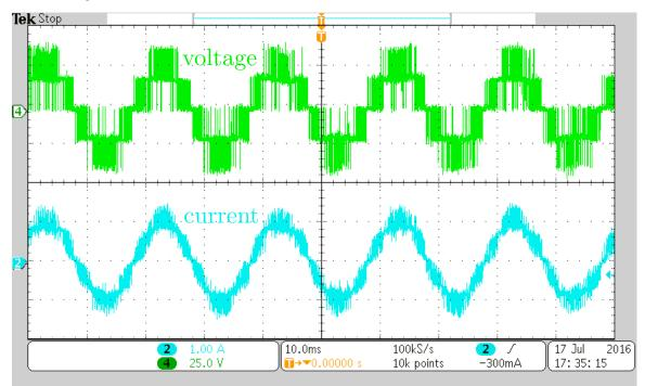
Figure 3.16. Converter's load-side waveforms in steady-state condition.
