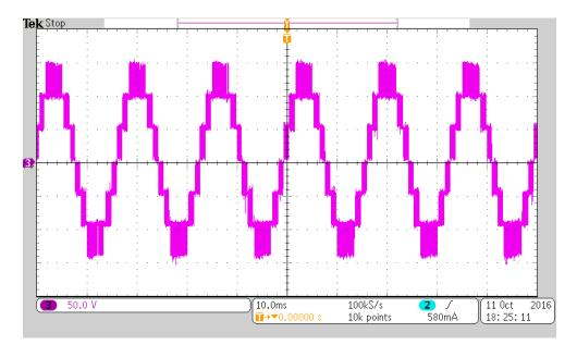
Figure 5.14. Converter's AC-side voltage in steady-state condition.
