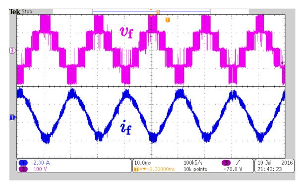
Figure 2.35. Converter's FB-side waveforms in steady-state condition.
