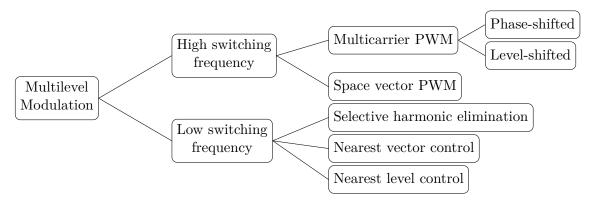
Figure 1.7. Classification of multilevel converter modulation techniques.
