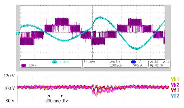
Figure 2.36. Dynamic response of the converter to the load change.
