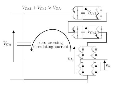
Figure 5.2. Zero-crossing circulating current in one phase of the converter.
