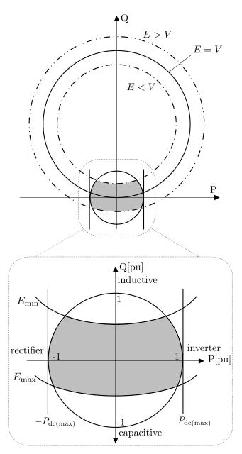
Figure 5.7. PQ chart of the converter considering VSC limitation.
