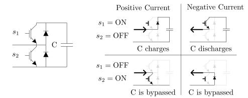
Figure 1.10. Capacitor charging/discharging based on HBSM's status.
