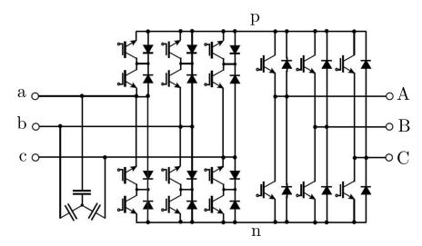
Figure 1.4. Conventional Indirect Matrix Converter.
