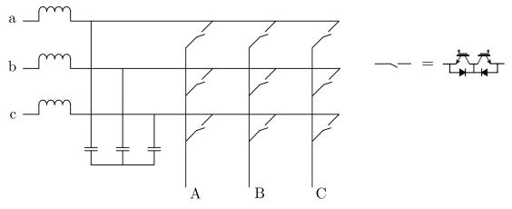
Figure 1.3. Conventional Direct Matrix Converter.
