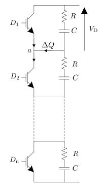
Figure A.4. Shunt capacitors for transient reverse blocking voltage.
