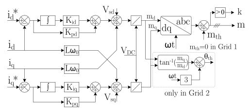
Figure 3.10. The schematic diagram of the current controller.
