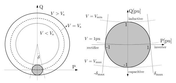
Figure 2.23. The power capability chart of SMMC.
