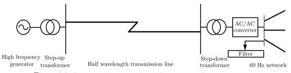
Figure 1.1. Schematic diagram of high-frequency half-wavelength line
