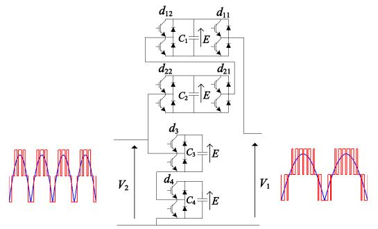
Figure 2.7. Schematic diagram of a 5-level SMMC leg.
