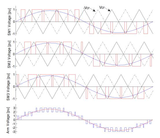
Figure 1.8. Multilevel phase-shifted carrier-based technique.
