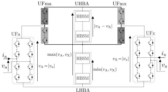
Figure 3.1. The schematic diagram of single-phase n-level MMMC.
