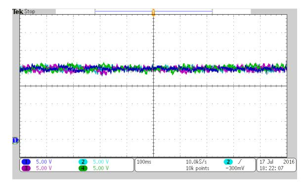
Figure 3.17. Capacitor voltages in steady-state condition.
