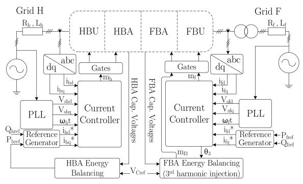
Figure 2.25. The schematic diagram of control strategy.
