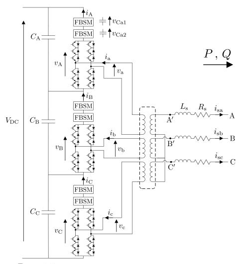
Figure 5.10. Schematic diagram of a 9-level SHMMC studied in MATLAB/Simulink.
