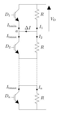
Figure A.2. Shunt resistors for voltage equalization in off-state.
