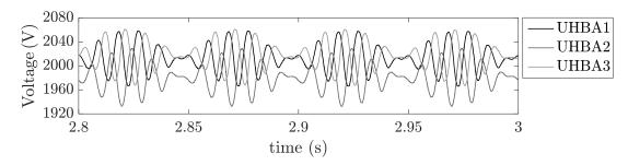
(a) Upper half-bridge arm capacitor voltages
