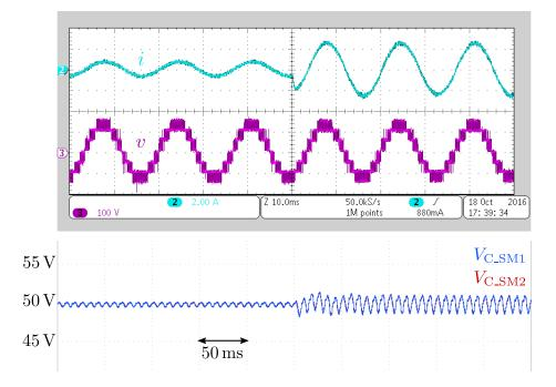
Figure 5.16. Dynamic response of the converter to the sudden load decrease.
