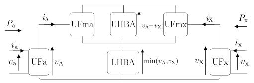
Figure 3.4. Simplified schematic diagram of a single-phase MMMC.
