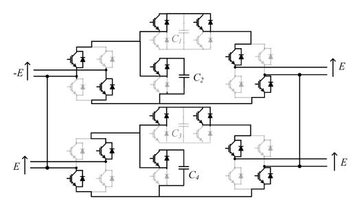
Figure 2.3. Shorting capacitor  $C_2$  without using isolating transformer.
