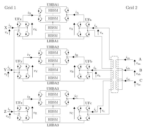
Figure 3.2. The schematic diagram of 3-phase MMMC.
