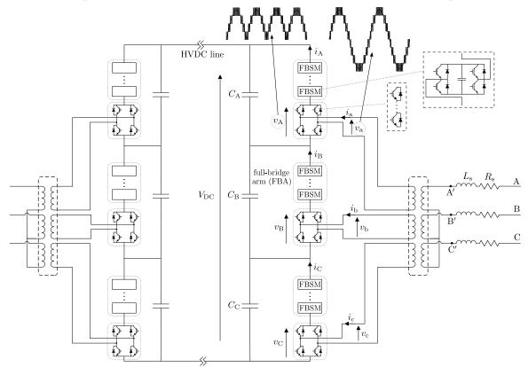
Figure 5.1. The schematic diagram of back-to-back SHMMC.
