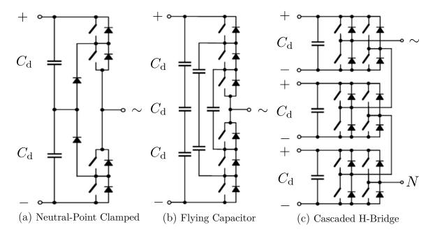
Figure 1.5. Different types of conventional multilevel converters.
