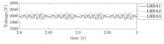
(b) Lower half-bridge arm capacitor voltages
