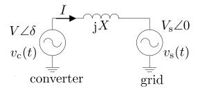
Figure 2.22. Simplified single-line diagram of converter-grid circuit.
