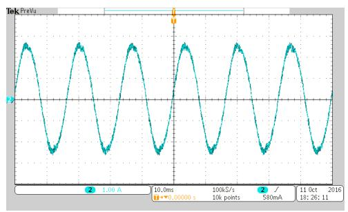
Figure 5.15. Converter's AC-side current in steady-state condition.
