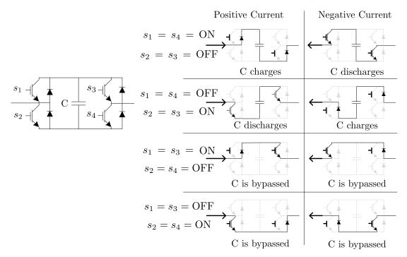
Figure 1.11. Capacitor charging/discharging based on FBSM's status.
