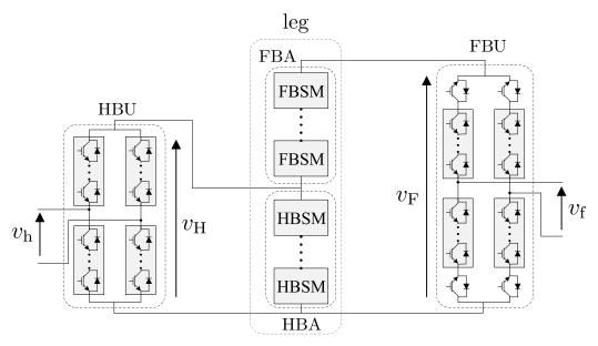
Figure 2.5. Schematic diagram of SMMC with modified FBU.
