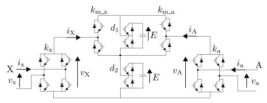
Figure 3.3. The schematic diagram of single-phase 3-level MMMC.
