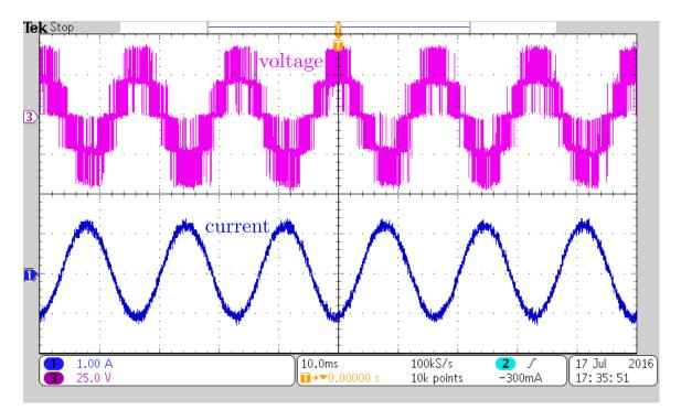
Figure 3.15. Converter's supply-side waveforms in steady-state condition.
