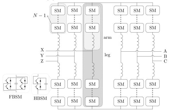
Figure 1.6. Three phase conventional B2B-MMC.
