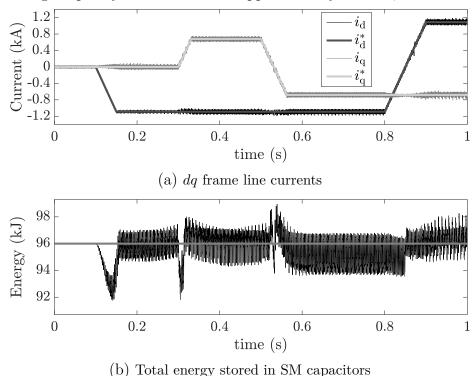
Figure 5.12. Transient simulation results.
