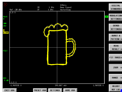
Fig. 1-17: I/Q diagram of a signal generated by a vector signal generator.
