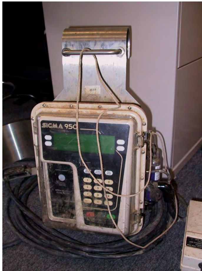
Figure 2. The flow meter that was used to measure the flow rate in the manhole.
