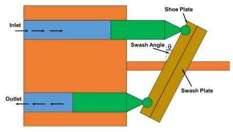
Figure 5.3.6 Swash plate piston pump
