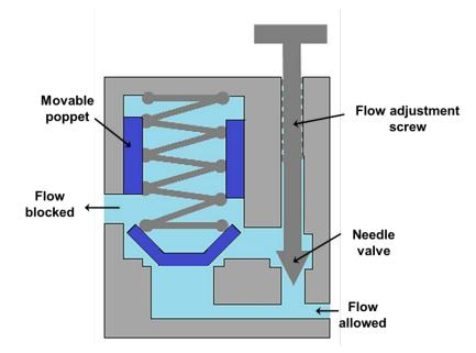
Figure 5.4.3 Restriction check valve
