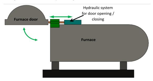
Figure 5.8.3 Furnace and its door
