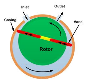
Figure 5.3.1 Schematic of working principle of vane pump
