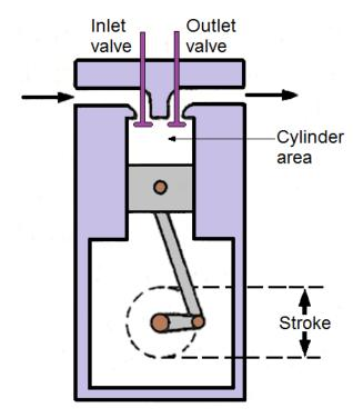
Figure 5.1.4 Reciprocating or positive displacement pump
