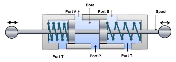
Figure 5.5.8 Two position four way DCV: P to A and B to T
