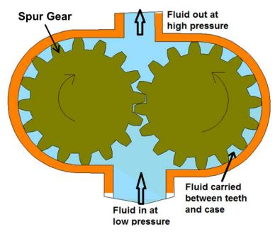
Figure 5.2.1 Gear pump
