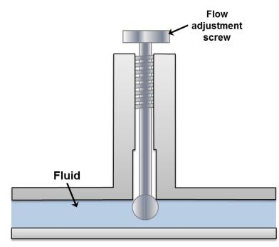
Figure 5.5.11 Flow Control Valve
