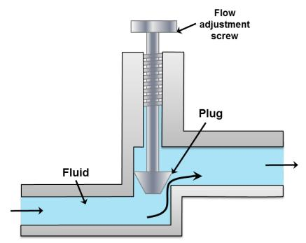
Figure 5.5.12 Plug or glove valve
