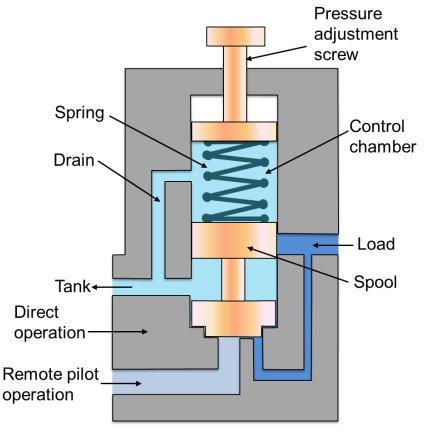
Figure 5.6.4 Counter Balance Valve
