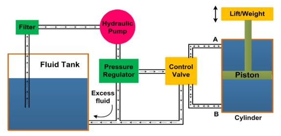
Figure 5.1.2 Schematic of hydraulic system
