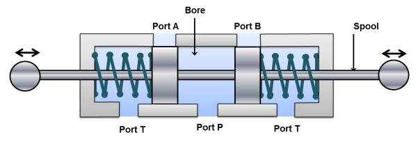
Figure 5.5.3 Three position four way valve: closed center
