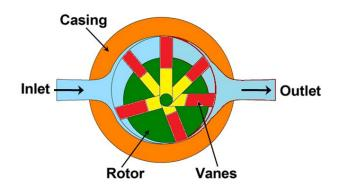
Figure 5.3.2 Unbalanced vane pump
