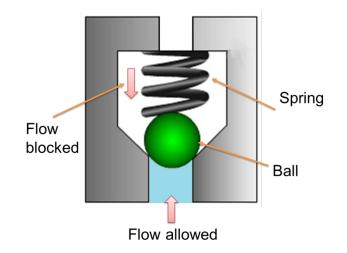
Figure 5.4.1 Inline check valve
