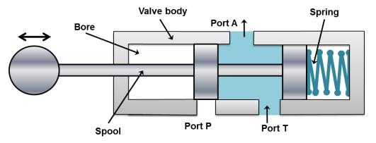
Figure 5.4.8 Three way valve in closed position
