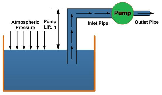
Figure 5.1.5 Pump lift
