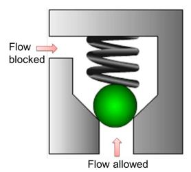
Figure 5.4.2 Right angle check valve
