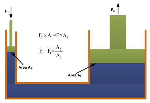
Figure 5.1.1 Principle of hydraulic system
