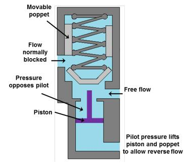
Figure 5.4.4 Pilot operated check valve
