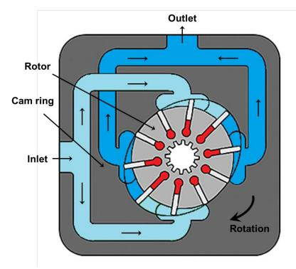
Figure 5.3.3 Balanced Vane Pump
