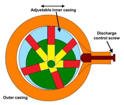
Figure 5.3.4 Adjustable vane pump
