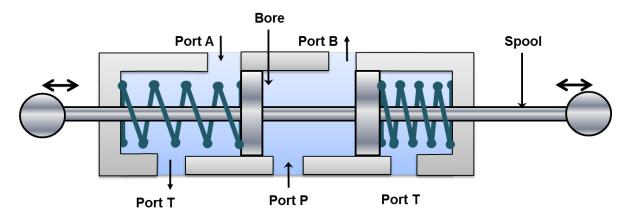
Figure 5.5.7 Two position four way DCV: P to B and A to T
