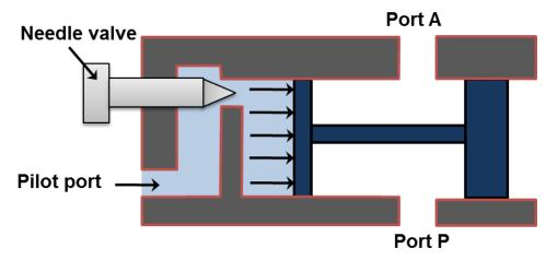
Figure 5.5.10 Pilot actuated DCV
