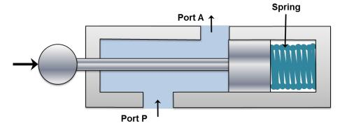
Figure 5.4.6 Valve opened by actuation
