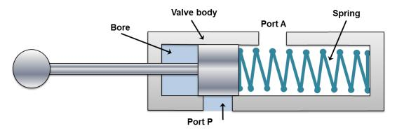
Figure 5.4.5 Valve closed
