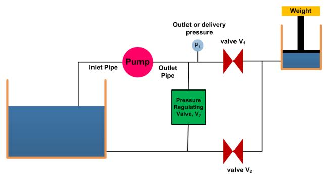
Figure 5.1.6 Schematic of pressure regulation
