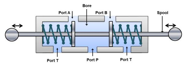
Figure 5.4.9 Three position four way valve in open center mode
