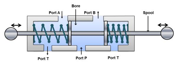
Figure 5.5.1 Three position four way valve: P to B and A to T
