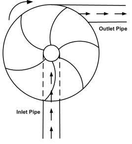
Figure 5.1.3 Centrifugal pump
