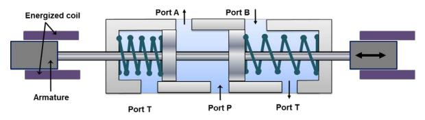
Figure 5.5.9 Working of solenoid to shift spool of valve
