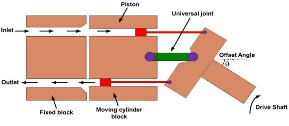
Figure 5.3.5 Bent axis piston pump
