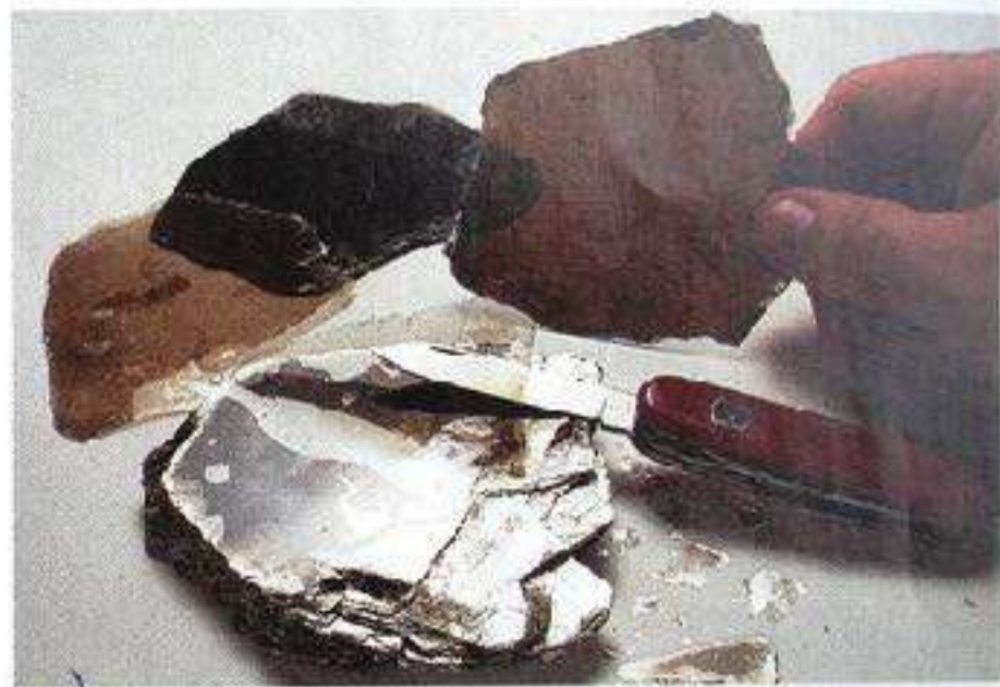
Figure 2.23 Cleavage of mica. The diagram shows the cleavage planes in the mineral structure, oriented perpendicularly to the plane of the page. Horizontal lines mark the interfaces of silica-oxygen tetrahedral sheets and sheets of aluminum hydroxide bonding the two tetrahedral layers into a "sandwich." Cleavage takes place between composite tetrahedral-aluminum hydroxide sandwiches. The photograph shows thin sheets separating along the cleavage planes. [Chip Clark.]
