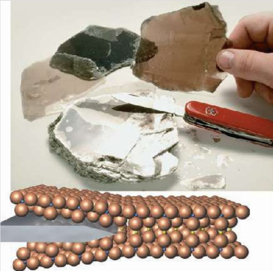
FIGURE 2.15 The thin sheets shown here were produced by splitting a mica (muscovite) crystal parallel to its perfect cleavage. (Photo by Chip Clark)
