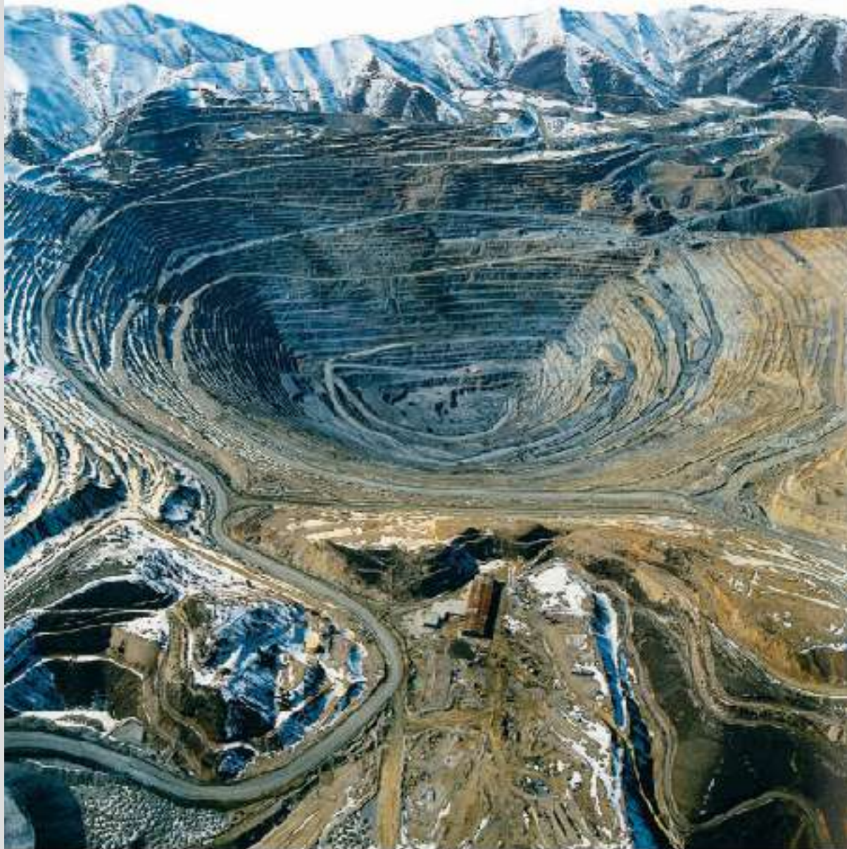
FIGURE 2.24 Aerial view of Brigham Canyon copper mine near Salt Lake City, Utah. Although the amount of copper in the rock is less than 1 percent, the huge volume of material removed and processed each day (about 2.5 million tons) yields enough metal to be profitable. (photo by Michael Laiter)
