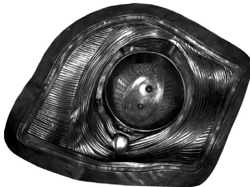
FIGURE 1.181 Model for the manufacture of an electroplated mold for the production of anatomical demonstration objects (e.g., eye)
