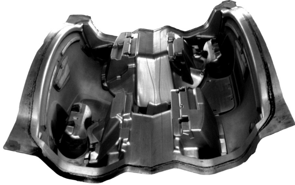
FIGURE 1.185 Shaping contour with double electroplated mold to produce two instrument panels at the same time
