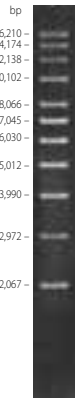
Supercoiled DNA Ladder 0.2 µg/lane; 0.9% agarose gel containing 2 µg/ml ethidium bromide. Cat. No. 15622012
