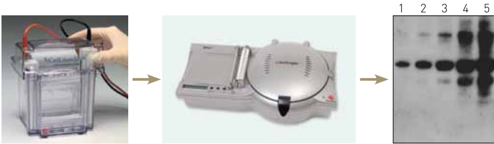
Figure 1. The Novex ® accelerated method provides a complete workflow solution from gels to blotting to detection, typically in 1 hour.
