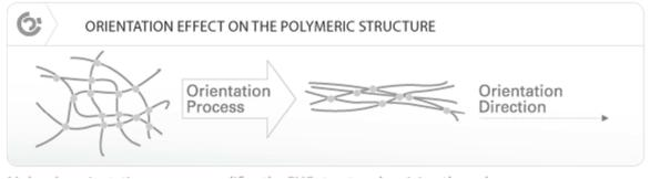
Figure 3 – Orientation Process
