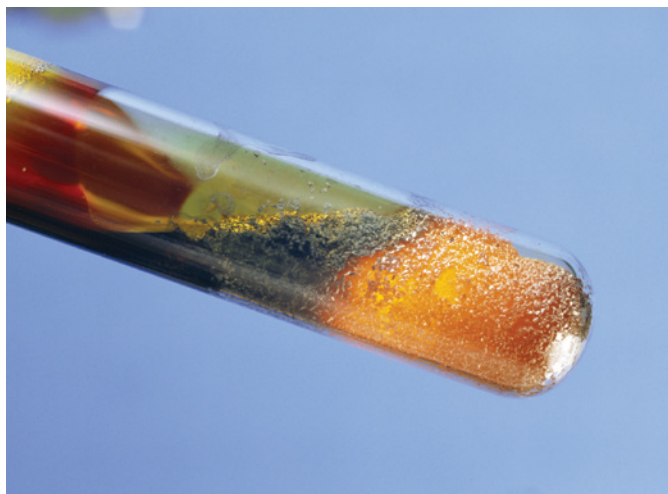
Figure 1.9 Iron reacting with sulfur to produce iron sulfide. We can calculate exactly how much iron is needed to react with sulfur and the mass of the products formed by knowing the molar mass of each reactant and the balanced chemical equation.
