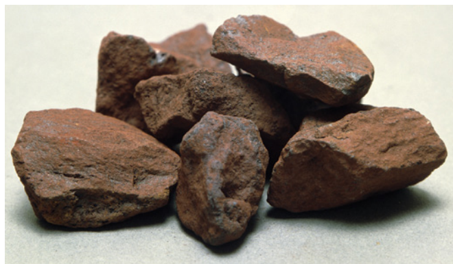
Figure 1.10 This iron ore is impure Fe 2 O 3 . We can calculate the mass of iron that can be obtained from Fe 2 O 3 by using molar masses.
