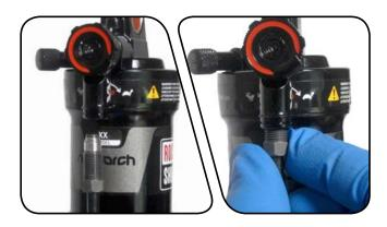
While continuing to push the hose into the rear shock banjo fitting, use a torque wrench with an 8 mm crowfoot socket to tighten the compression nut to  $5 \text{ N} \cdot \text{m}$  (44 in-lb).
