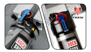
6 If the shock is collapsed so that a minimal amount of damper body is visible, there is still air pressure in the air can.
