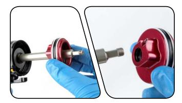
Use a pick to remove and replace the internal seal o-ring located in the internal seal gland.
