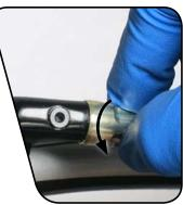
**3** Use a T10 TORX<sup>®</sup> wrench to thread the remote bleed screw into the bleed port.
