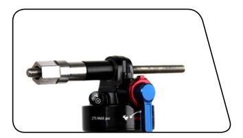
Thread the large, open end of the catcher onto the rod until it rests on the eyelet.
