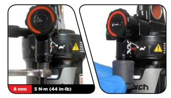
Cutting the hose introduces air into the system. It is necessary to bleed the remote assembly for optimal performance. See <u>XLoc Full</u> <u>Sprint<sup>™</sup> Bleed Procedure</u> for instructions.
