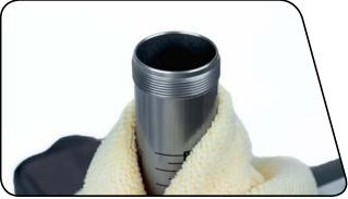
Pour new RockShox 3wt suspension fluid into the damper body until it is level with the top.
