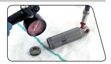
Spray isopropyl alcohol on the inside and outside of the damper body and clean it with a rag.
