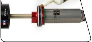
2 Apply a small amount of grease to the air can threads. Position the threaded side of the air can over the damper body eyelet.
