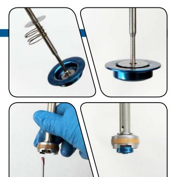
Test the compression rod and top hat function by rotating the compression lever to the closed position and pushing on the top hat. The top hat should have a small amount of movement. If it does not move, adjust the top hat spring so it is seated inside the groove.
