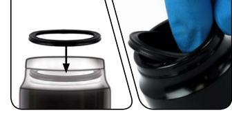
6 Install the second backup ring by inserting one end into the air can, then push the remainder of the ring into the can, so that it rests on the quad seal at the top of the second deepest groove.
