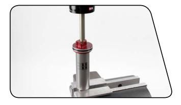
Use a 2 mm hex wrench to remove the bleed screw, located in the seal head/air piston.
