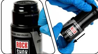
High Volume Air Cans: Use your fingers to remove and replace the 10 High volume sleeve o-rings.
