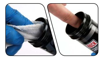
Install the first backup ring by inserting one end into the air can, then push the remainder of the ring into the can, so that it rests on the bottom of the second deepest groove.
