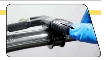
**2** To replace the hydraulic hose: Slide the hose boot off the rear shock banjo fitting.
