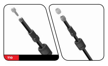
Push the hose into the rear shock banjo fitting until it stops.
