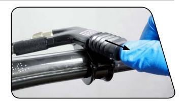
Gently pull up on the remote syringe plunger to remove any remaining air bubbles from inside the remote, then push on the plunger to force fluid into the remote. Repeat this process until no more air bubbles transfer into the syringe.
