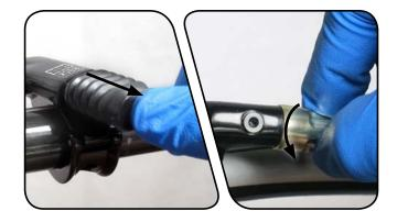
2 Use a T25 TORX<sup>®</sup> wrench to loosen the clamp bolt and rotate the remote on the handlebar until the bleed screw is at the highest point.
