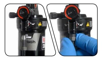
While continuing to push the hose into the rear shock banjo fitting, use a torque wrench with an 8 mm crowfoot socket to tighten the compression nut to 5 N·m (44 in-lb).
