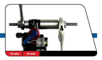
Reinsert the threaded rod and push pin through the shaft eyelet. Thread the large, open end of the catcher along the rod until it rests against the shaft eyelet.
