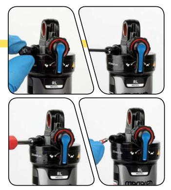
Use a Schrader valve tool to remove the damper air fill port cap. Use a small hex wrench or pick to depress the Schrader valve and release all air pressure from the damper.
