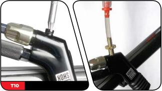
While holding both syringes upright, push on the rear shock syringe plunger and pull up on the remote syringe plunger at the same time. This will force fluid and any air bubbles through the hose and into the remote syringe. Continue to push on the rear shock syringe plunger until the syringe is nearly empty.
