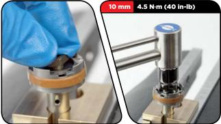
Install the top hat spring and top hat washer onto the compression rod. Hold the compression rod vertically so the spring is seated in the groove inside the top hat.
