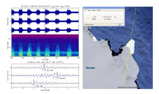
Figure 24: Left: Close-up of broadband (3 Hz to 103 Hz) pressure time series and spectrogram at  $20:42:27 \pm 300$  s on 14 May 2011 for Cape Leeuwin; lower graph shows time lag plot indicating sound originates from bearing 165 deg. Right: Ice tongue on Antarctica at bearing 165.
