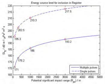
Figure 2: Energy source level threshold [dB re 1 µPa<sup>2</sup> m<sup>2</sup> s] vs significant impact range [m].
