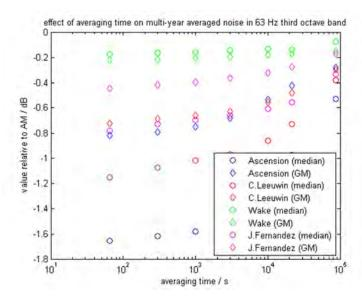
Figure 33: Differences  $L_G$  –  $L_A$  and  $L_M$  –  $L_A$  vs snapshot duration for four CTBTO sites; change seems to accelerate (increase in slope) for T > 1 hour; at least for Cape Leeuwin and Ascension Is. colours: Ascension Island, Cape Leeuwin, Wake Island, Juan Fernández.
