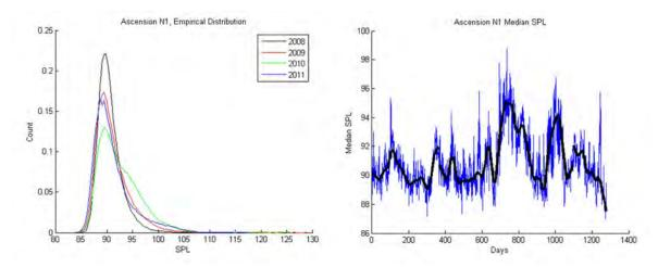
Figure 19: Left graph: Histogram of  $SPL_{63}$  distribution for Ascension Island (T = 65.5 s); right graph: daily median of  $SPL_{63}$  vs time.
