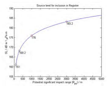
Figure 3: Source level threshold [dB re 1 µPa m] vs significant impact range for sonar [m].
