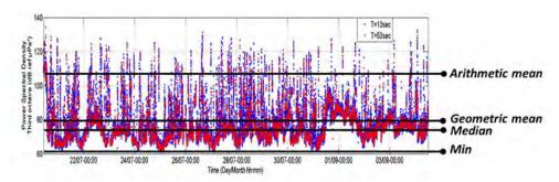
Figure 1: Example of approx. 14 days of continuous measurement in the 125 Hz third octave band made off Cork harbour (Ireland) entrance made during the STRIVE project (source: Quiet-Oceans).
