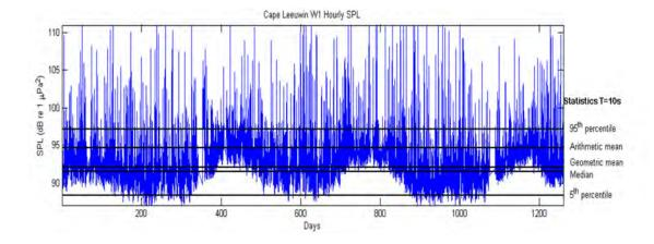
Figure 3: Example of 3 years of measurements in the 63 Hz third octave band made at the CTBTO Cape Leeuwin station.
