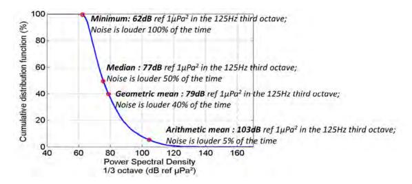
Figure 2: Statistical representation of the measured sound pressure level in the 125 Hz third octave band off Cork harbour as a cumulative distribution function, the exceedance<sup>12</sup>.
