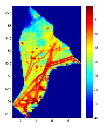
Figure 8: Distribution of shipping density  $10\log_{10}(25\ N/\mathrm{km^2})$  where N is the average areic shipping density in 2007 (data obtained from IMARES).
