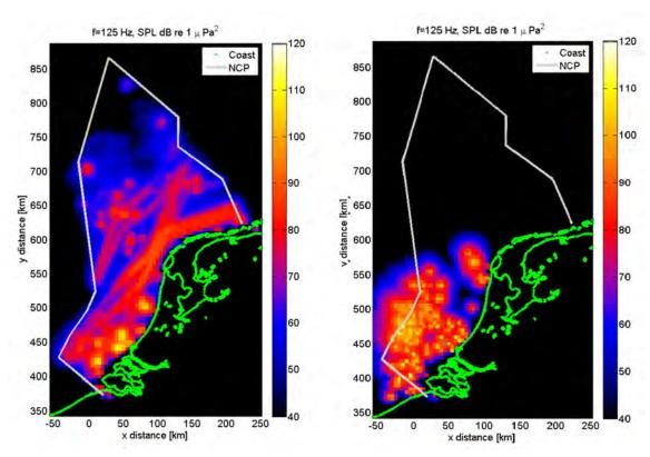
Figure 12: Annually averaged noise predictions for the Dutch North Sea: SPL in the decidecade centred at 125 Hz. Left: shipping noise for 2007; right: noise from explosions, averaged over two years (2010 and 2011). Receiver depth is 1 m. (provided by Özkan Sertlek (University of Leiden) and TNO, © Özkan Sertlek).
