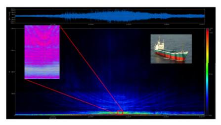
Figure 15: Spectrogram of passing ship, CPA at 0.3 nmi (@DW ShipConsult)
