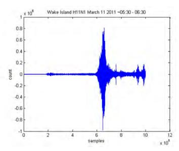
Figure 30: Broadband pressure signature on H11 (Wake Island) caused by Tohoku earthquake on 11 March 2011. The maximum sound pressure magnitude corresponds to a sound pressure of -550 Pa (- $10^6$  counts, with a sensitivity of 1.83 counts per millipascal).
