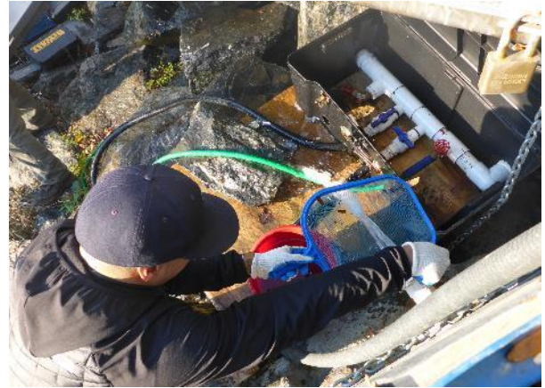
Photo 24: The knife valve is open to allow the water to flow out of the holding tank
