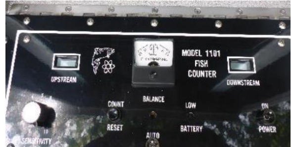
Photo 17: Fish counter device connected to tunnel
