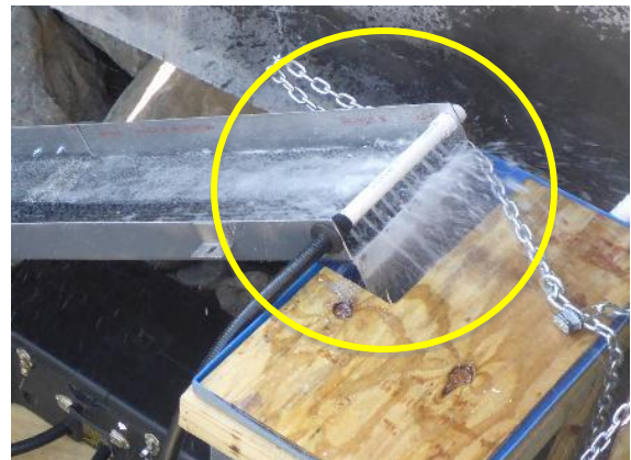
Photo 26: The upper spray bar's water pressure should be high enough to supply water to the passage and holding tank while still allowing eels to safely and efficiently climb up the ramps (yellow circle)
