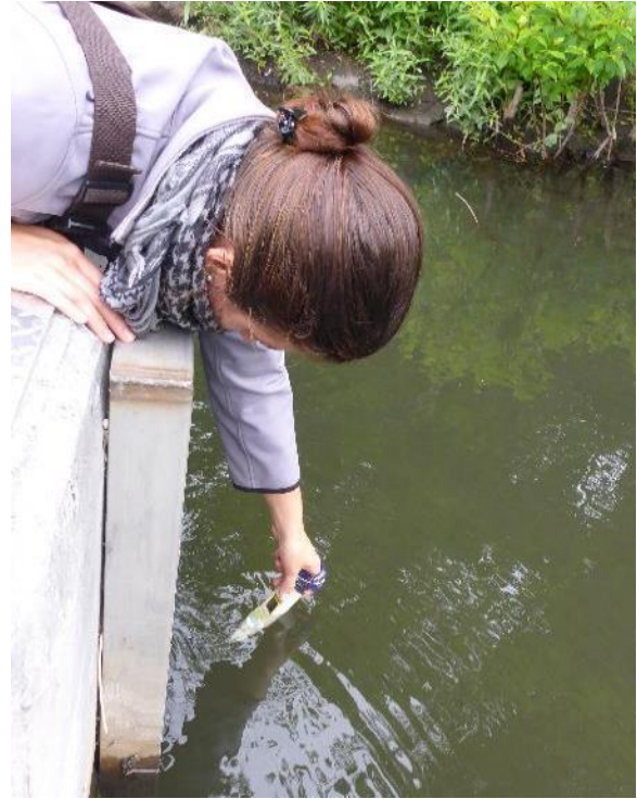
Photo 13: Collecting water temperature data at the exitway of the fish ladder
