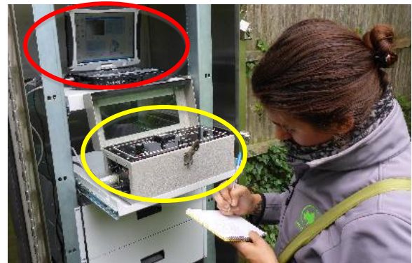
Photo 18: Fish counter device (yellow circle); underwater video camera is connected to laptop (red circle)
