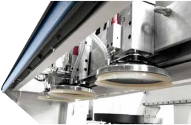
Precise and rapid panels positioning on the work table with a dedicated suction cups system.
