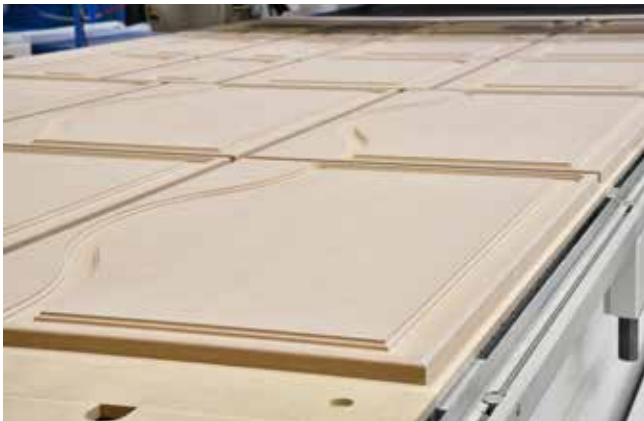
Optimal work piece holding with the high capacity vacuum up to 1000 m 3 /h.
