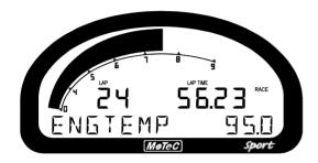
The alarms remain active until they are acknowledged, either by a driver activated switch or automatically after a defined period of time.
