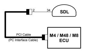
To connect a PC to the ECU disconnect the Computer Interface Cable from the SDL and attach it to the PC.
