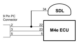
Note that Older M4 ECUs require a different connection method Note that the data to the SDL will be interrupted while a PC is connected. MoTeC Appendices 55
