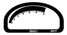
The 70 segment bar graph has a user definable range and is typically used as a tacho, however it can be used to display any other value. When used as a tacho it may be configured for up to 19,000 RPM.
