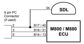
Note that the data to the SDL will be interrupted while a PC is connected (DOS software only)
