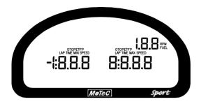
The three numeric displays (Left, Right and Top Right) can be programmed to display any value.
