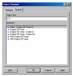
This method is most useful when selecting a channel from the available channels. For example, if 'Engine Temperature' has been assigned to an input pin, it can be easily located in the Search list, since this list normally only contains 50 to 100 items.
