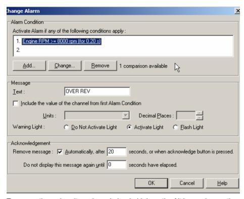
To access the various items in a window hold down the Alt key and press the key corresponding to the underlined letter of the item of interest, for example to select the 'Flash Light' item press Alt F
