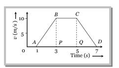
Solution: (b) Distance covered in total 7 seconds = Area of trapezium  $ABCD = \frac{1}{2}(2+6) \times 10 = 40 \text{ m}$
