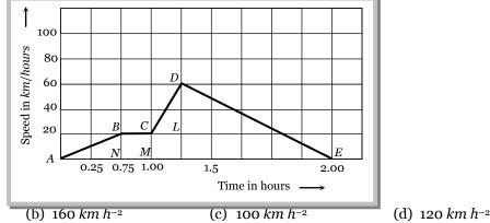
Solution: (b) Maximum acceleration means maximum slope in speed – time graph.
