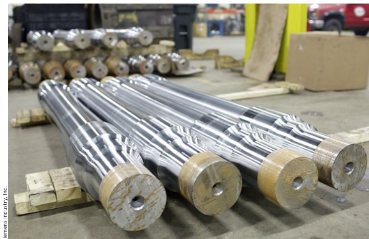
Raw hammer forged axles weigh approximately 2,200 lbs
