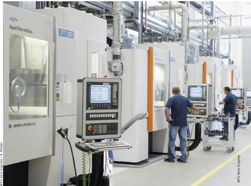
MTU Aero Engines uses identical high-performance five-axis milling centers for its new blisk production plant in Munich
