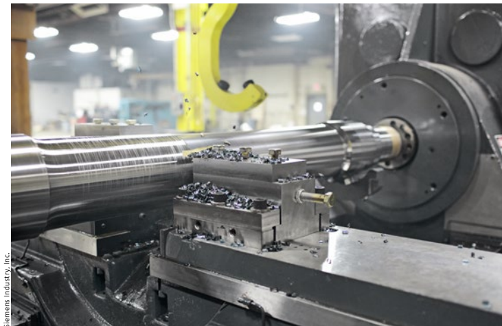
Semifinished axles are sent to the centerless grinding application before wheels are mounted
